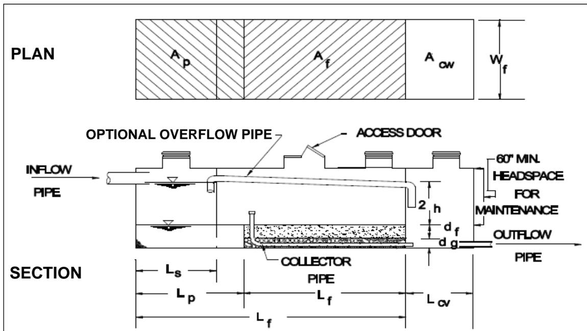
**Figure 12.6. D.C. Sand Filter – Cross Section**
