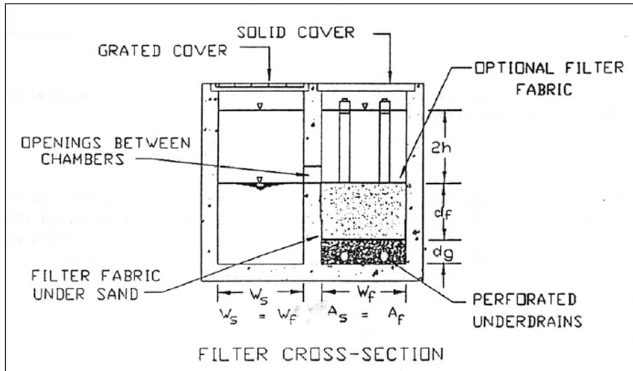
**Figure 12.7. Delaware Sand Filter – Cross Section**
