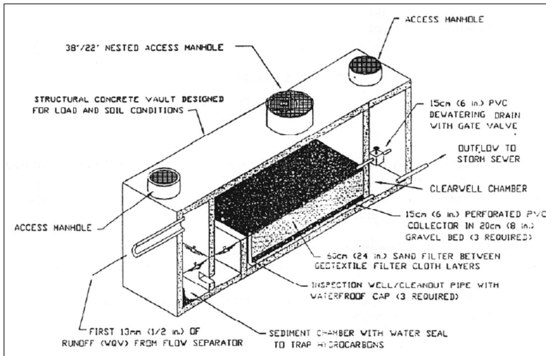
**Figure 12.1. Washington D.C. Underground Vault Sand Filter**
