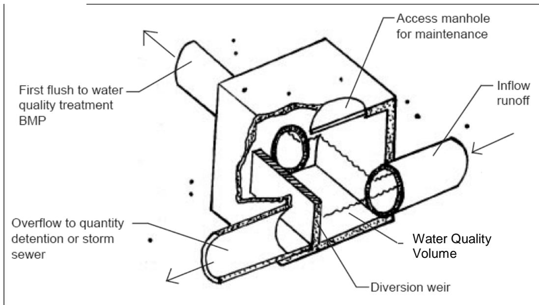
**Figure 12.4. Flow-splitting Diversion Weir (Bell, Warren, 1993)**
