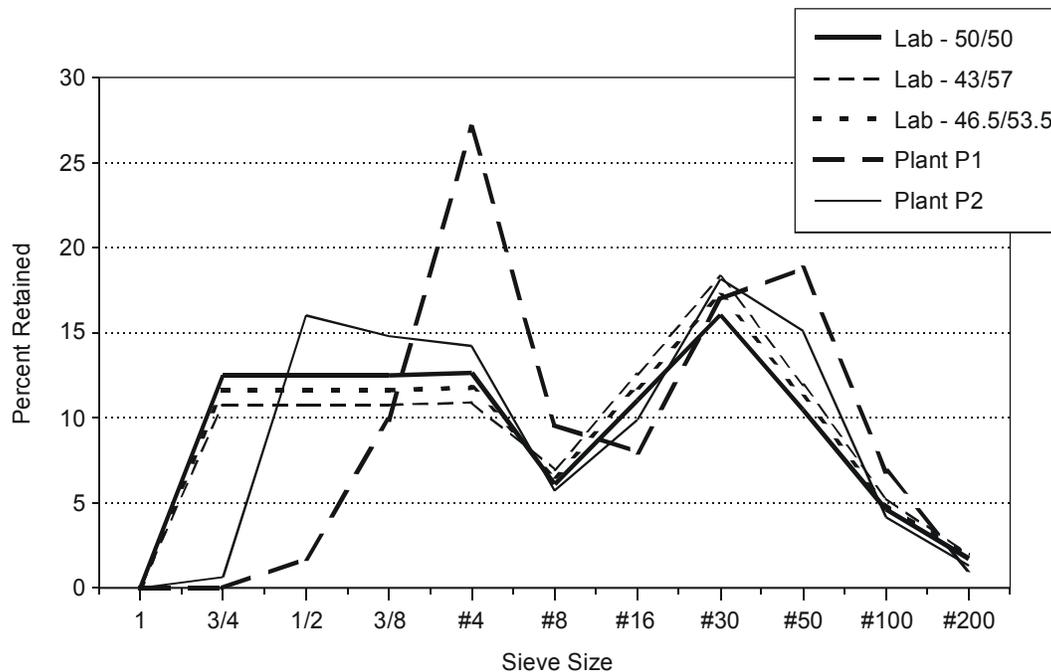
Figure 1. Aggregate Grading for Laboratory and Plant Phases (1 in = 25.4 mm)
