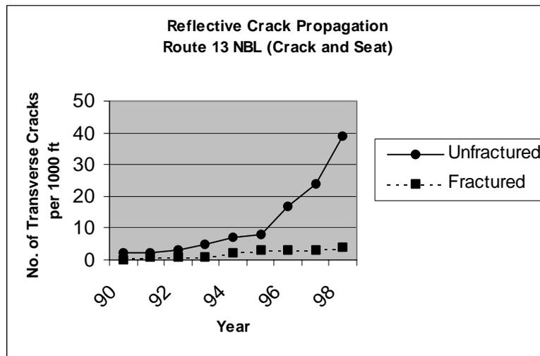
Figure 1. Reflective Cracking Over Time for Site 1, Unreinforced Concrete Slabs
