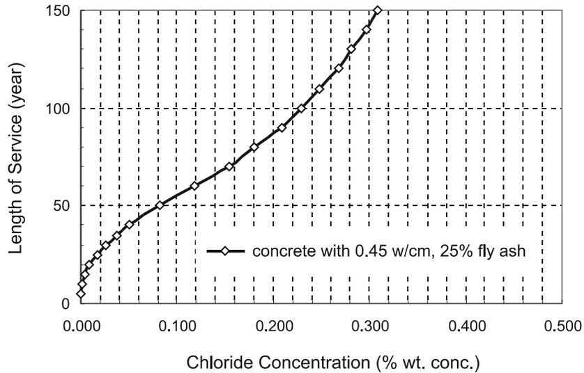
**Figure 1. Length of Service Required for Chloride Ions at the Depth of Top-Mat Bars (2.75 in) to Reach a Given Concentration in the Hypothetical Concrete Deck (0.025% Cl by weight of concrete = 1.00 lb/yd<sup>3</sup>)**
