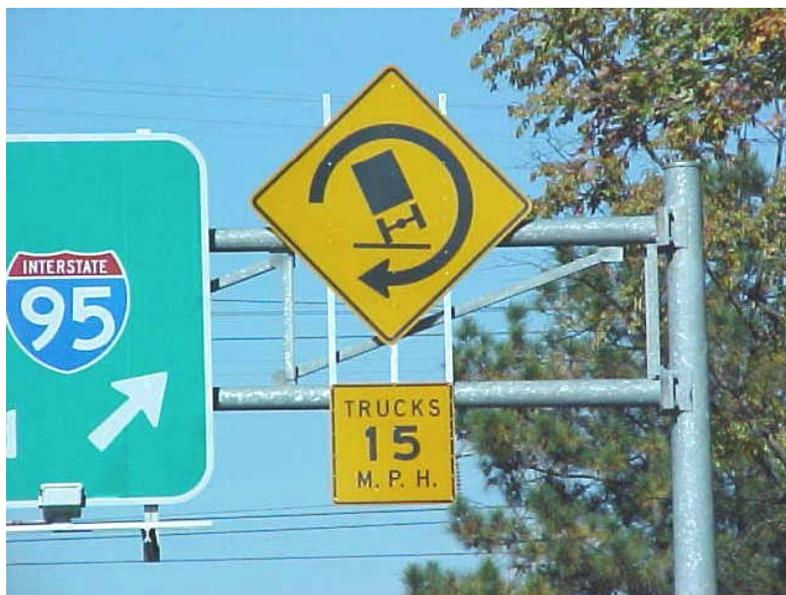
**Figure 2. Static Truck Rollover Sign**
