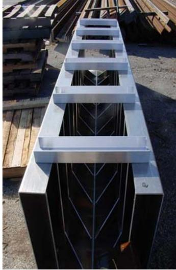
**Figure 8. Alaskan steep pass section built for Claiborne Run site.**
