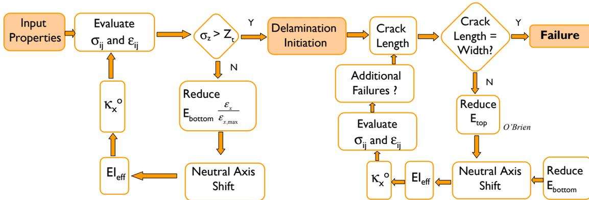
**Figure 9.** Flowchart of stress analysis and stiffness reduction, delamination determination, and stress redistribution following delamination.
