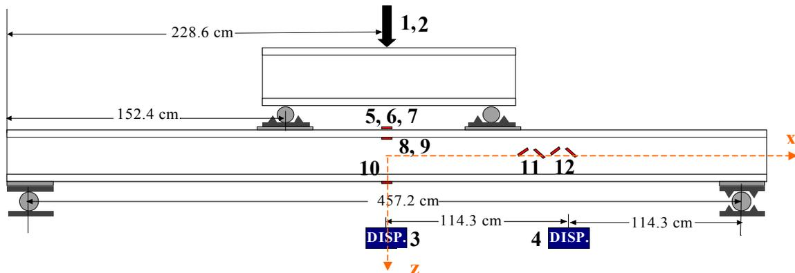
**Figure 6.** Schematic for the instrumentation used in the characterization of strength and fatigue. 1. Actuator Load, 2. Actuator deflection, 3. Mid-span Deflection, 4. Quarter Point Deflection, 5. Top Center Bending Strain, 6. Top Right Bending Strain, 7. Top Left Bending Strain, 8. Top Right Flange Bending Strain, 9. Top Left Flange Bending Strain, 10. Bottom Center Bending Strain, 11. Shear Strain 1 in outside of the constant moment region, 12. Torsional Strain at the  $\frac{1}{4}$  point.
