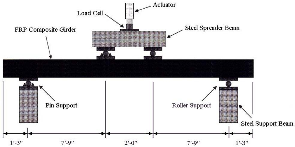
**Figure 5.** Schematic of four-point strength and stiffness setup.
