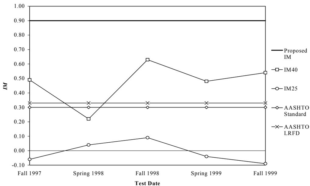
**Figure 11.** IM values based on mid-span strain data.
