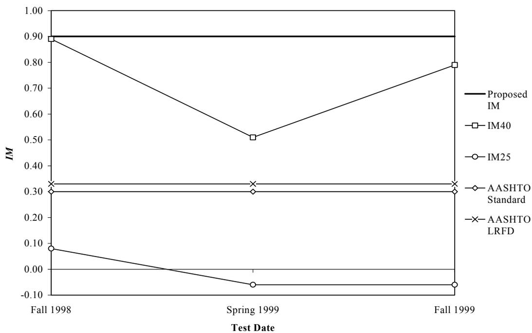
**Figure 12.** IM values based on mid-span deflection data.
