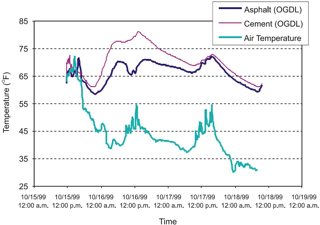
**Figure 2. Temperature Data for First 72 Hours for 12-ft Lane. The temperature sensor was close to the top surface of the pavement.**
