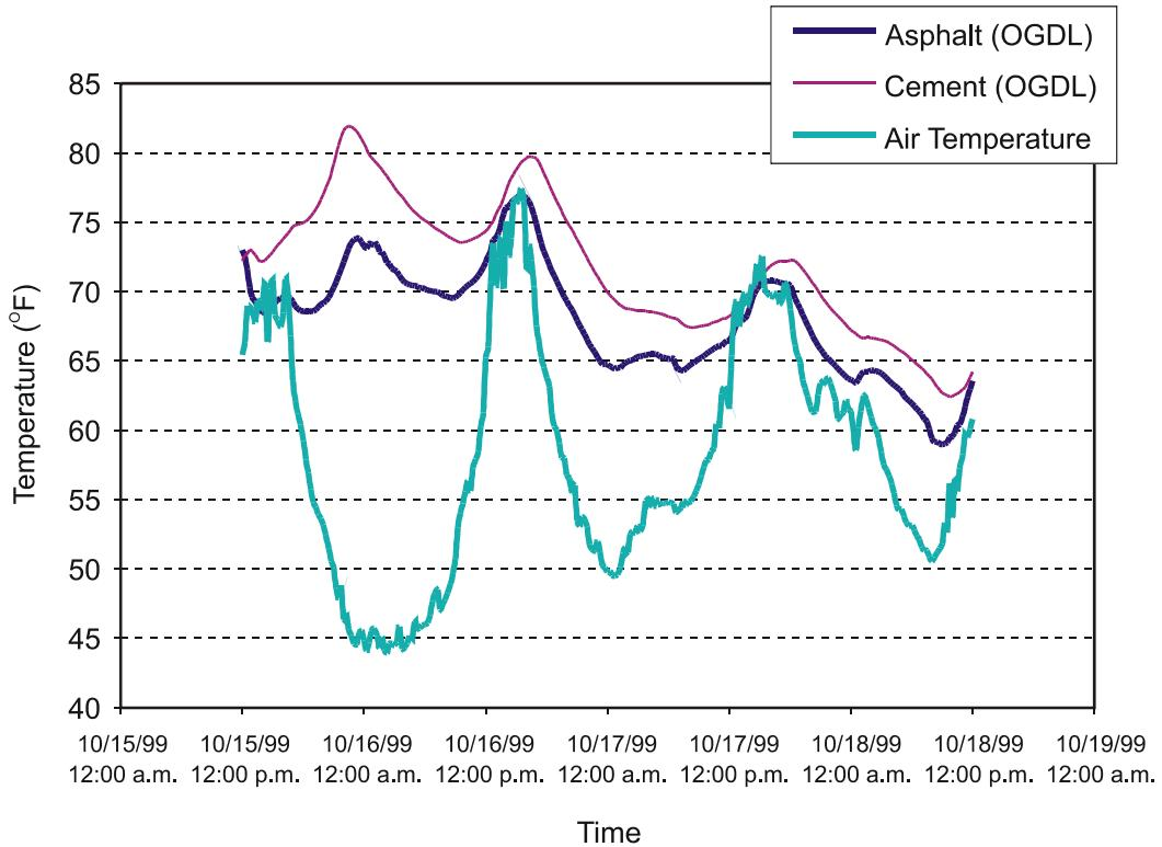
**Figure 1. Temperature Data for First 72 Hours for 14-ft Lane. The temperature sensor was close to the top surface of the pavement.**
