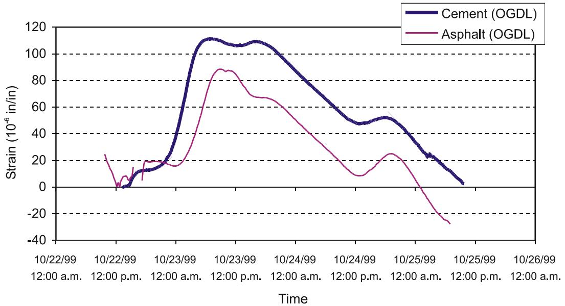
**Figure 5. Strain Data for Bottom Section of Slab for 12-ft Lane.**
