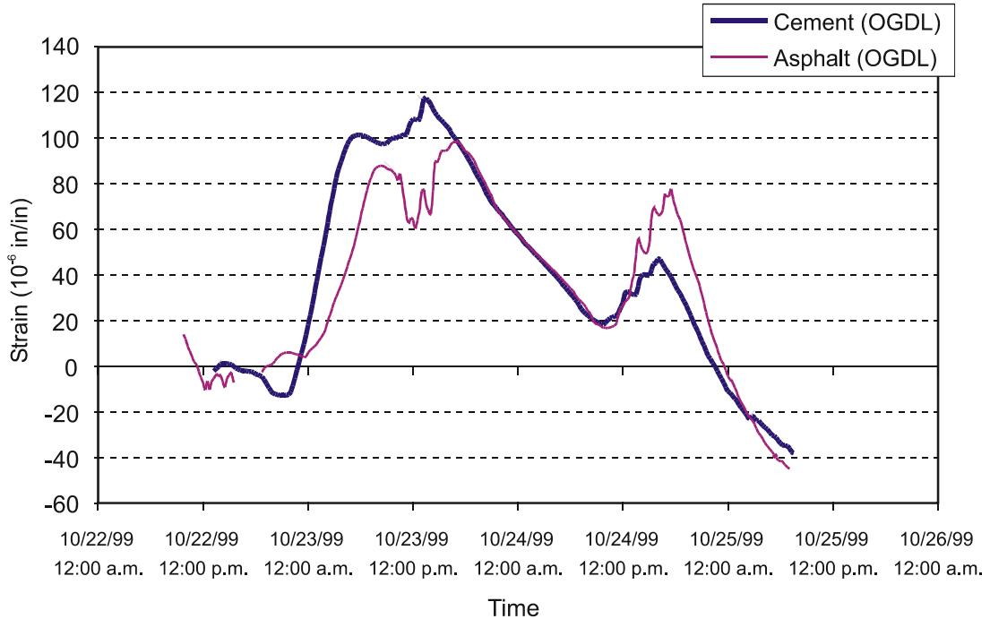
**Figure 4. Strain Data for Top Section of Slab for 12-ft Lane.**
