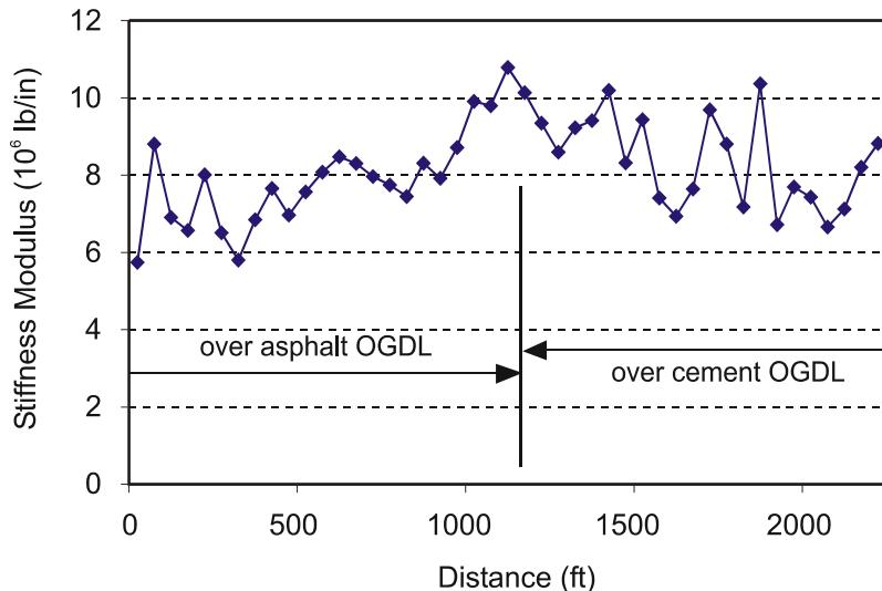
**Figure 6. FWD Data for Eastbound Lanes (12-ft lane).** The load was 16,000 lb; the average total pavement stiffness over the asphalt-stabilized OGDL was  $7.86 \times 10^6$  lb/in and over the cement-stabilized OGDL was  $8.42 \times 10^6$  lb/in.
