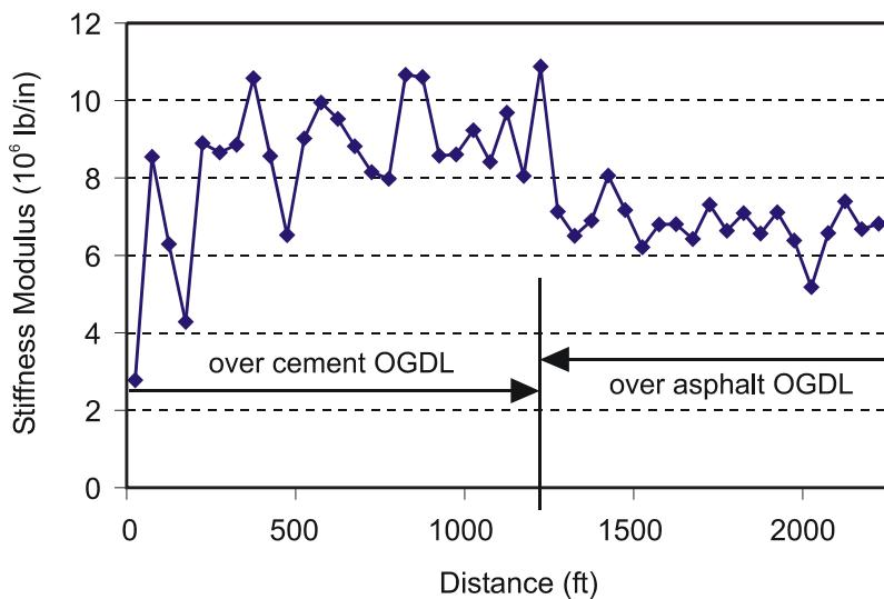
**Figure 7. FWD Data for Westbound Lanes (14-ft lane).** The load was 16,000 lb; the average total pavement stiffness over the asphalt-stabilized OGDL was  $7.03 \times 10^6$  lb/in and over the cement-stabilized OGDL was  $8.40 \times 10^6$  lb/in.
