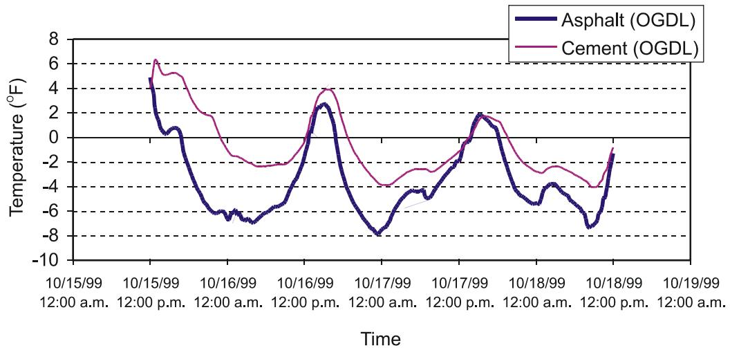
**Figure 3. Temperature Gradient for First 72 Hours Between Top and Bottom of Slab in 14-ft Section.**
