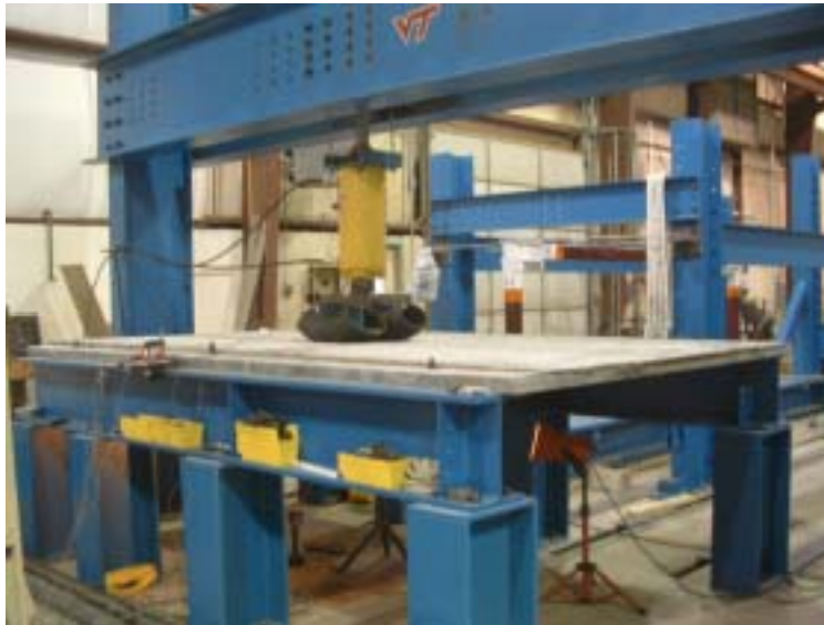
Figure 21. Tire Patch Used to Load Large Slabs.
