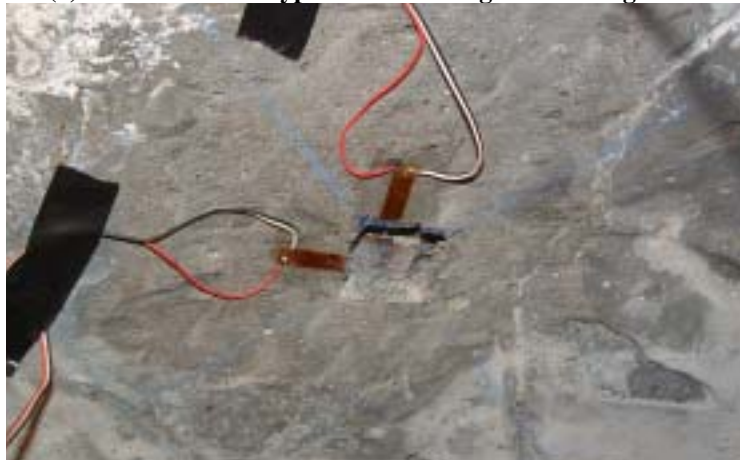
(a) Tensile Face of Typical Slab Failing in Punching Shear
