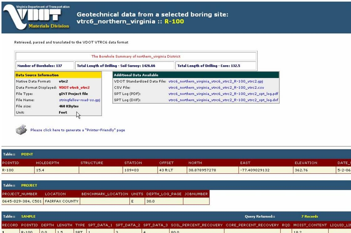
Figure 5. Example of Adaptive Translation of VTRC6-series Borehole Data
