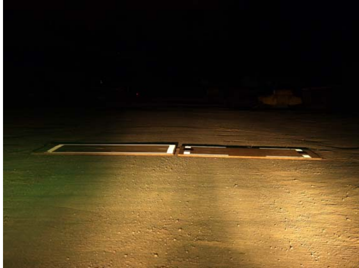
Figure 4. Outlined Plate and Corners Only Plate Under Low-Beam Headlights Zoomed in From 80 Feet
