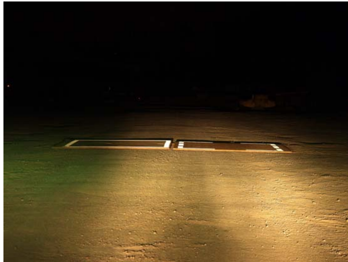
Figure 2. Outlined Plate and Corners and Skip Lines Plate Under Low-Beam Headlights Zoomed in from 80 Feet
