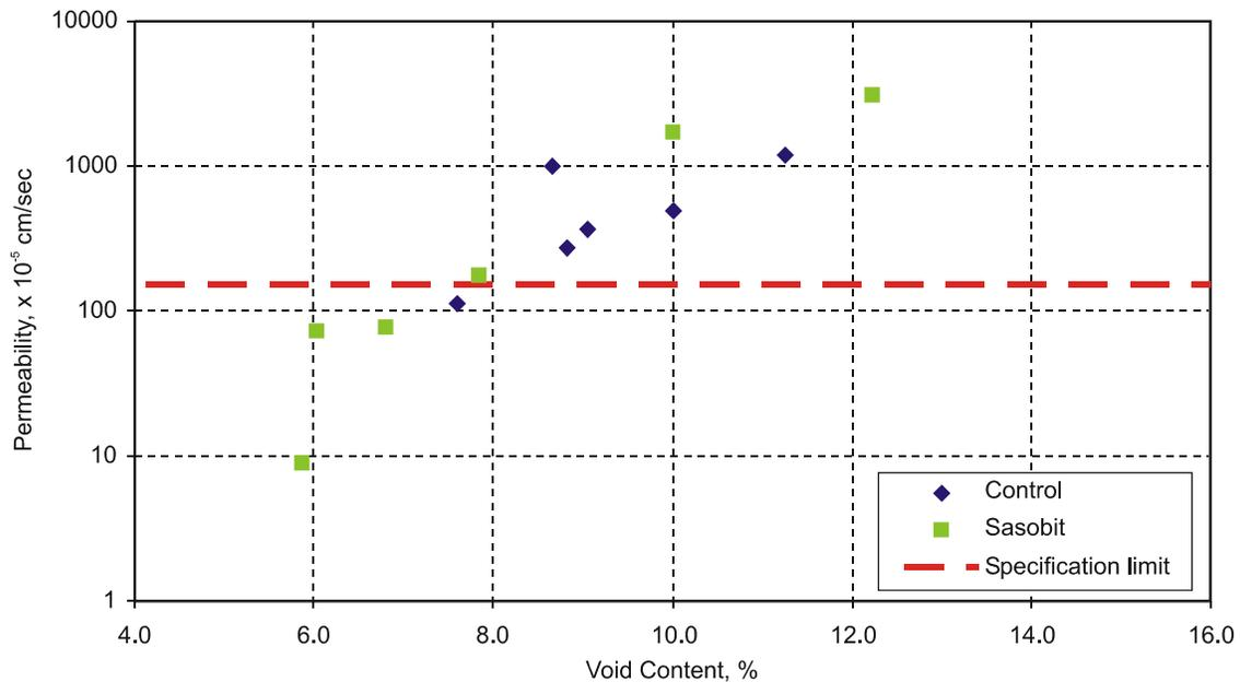
**Figure 11. Permeability Results for Trial B**
