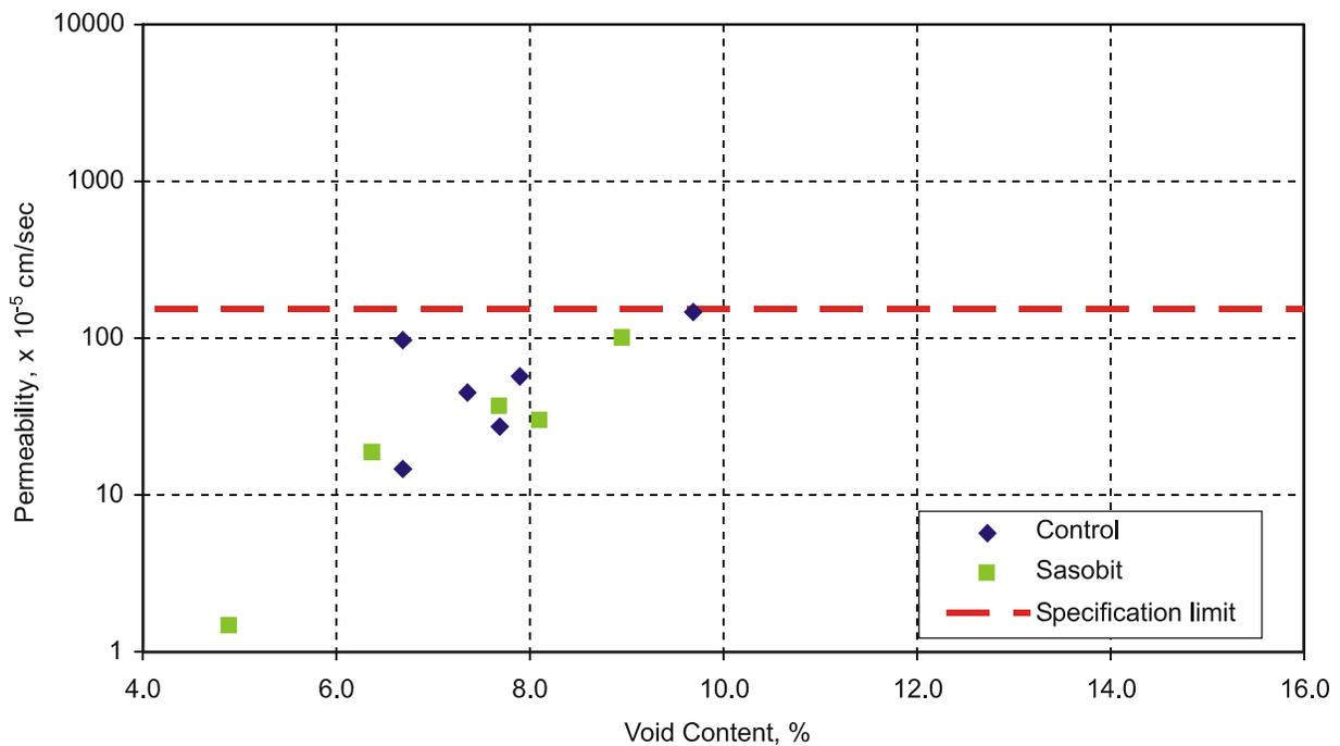
Figure 7. Permeability Results for Trial A
