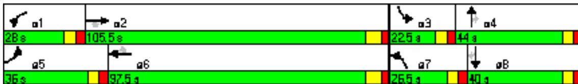
Figure 7. Intersection 12 Phase Diagram and Timings of Lead-Lead Phase Configuration
