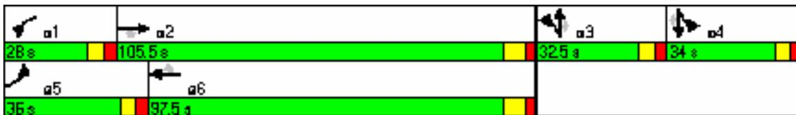
Figure 8. Intersection 12 Phase Diagram and Timings of Lead-Lag Phase Configuration
