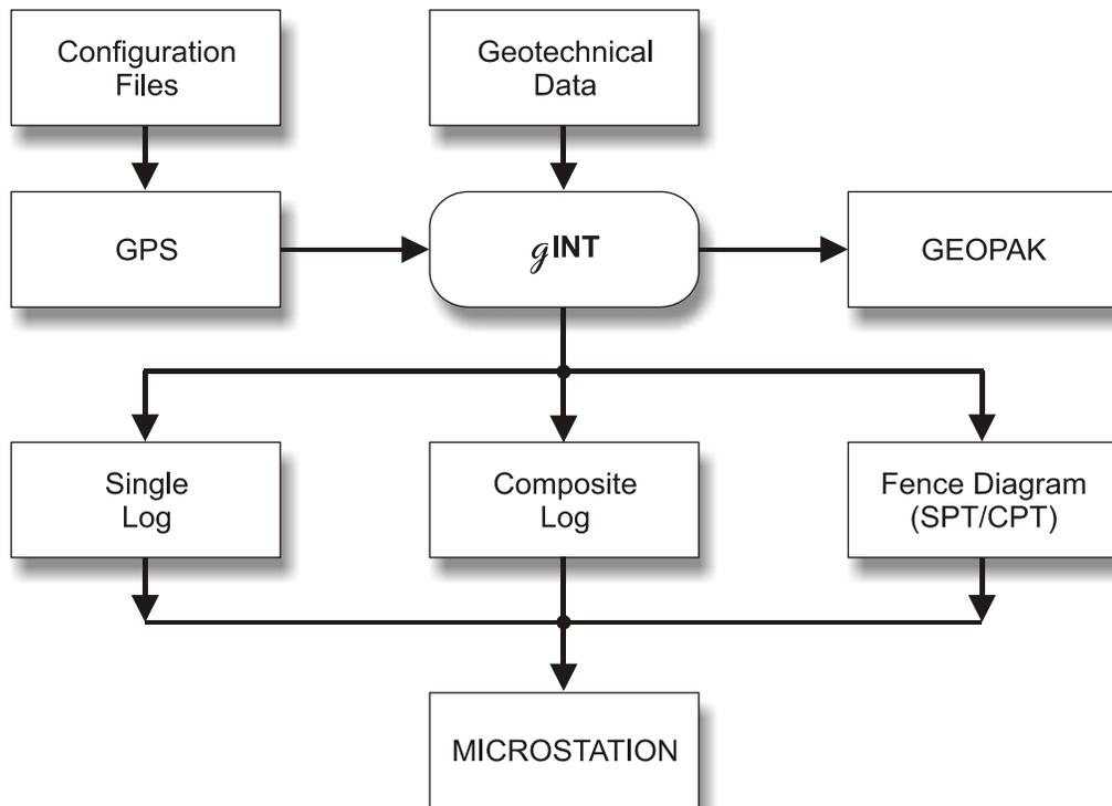
Figure 1. Geotechnical Data Processing at VDOT
