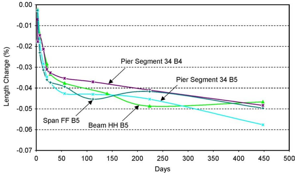
**Figure 2. Pamunkey Length Change Data for Steam-Cured Specimens**
