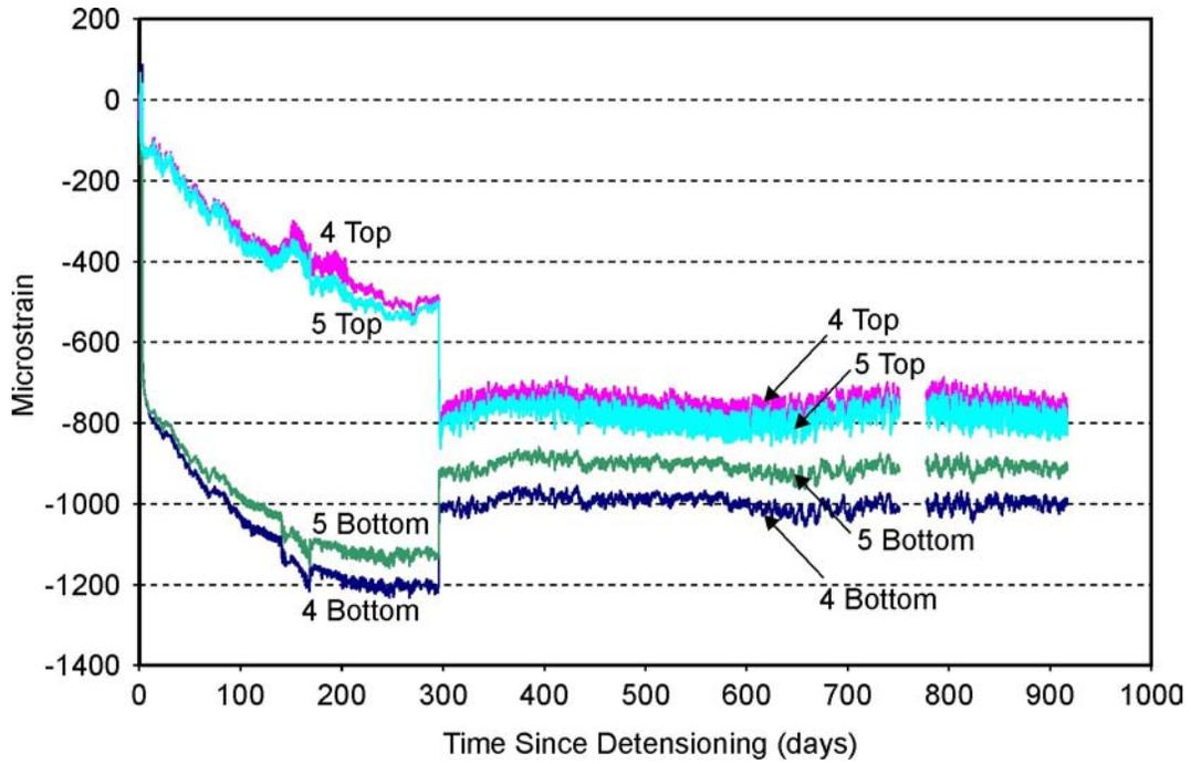
Figure 9. Strain Data for Span I Interior Beams of Mattaponi Bridge
