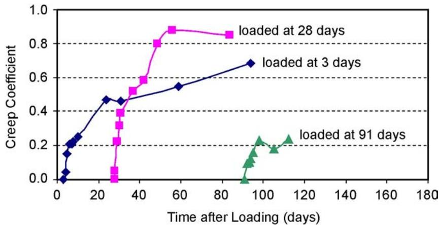
Figure 6. Creep Data for Pamunkey Bridge Beams
