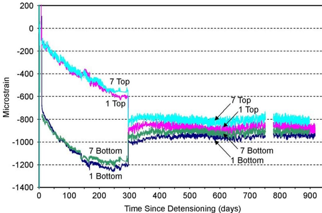
Figure 8. Strain Data for Span I Exterior Beams of Mattaponi Bridge
