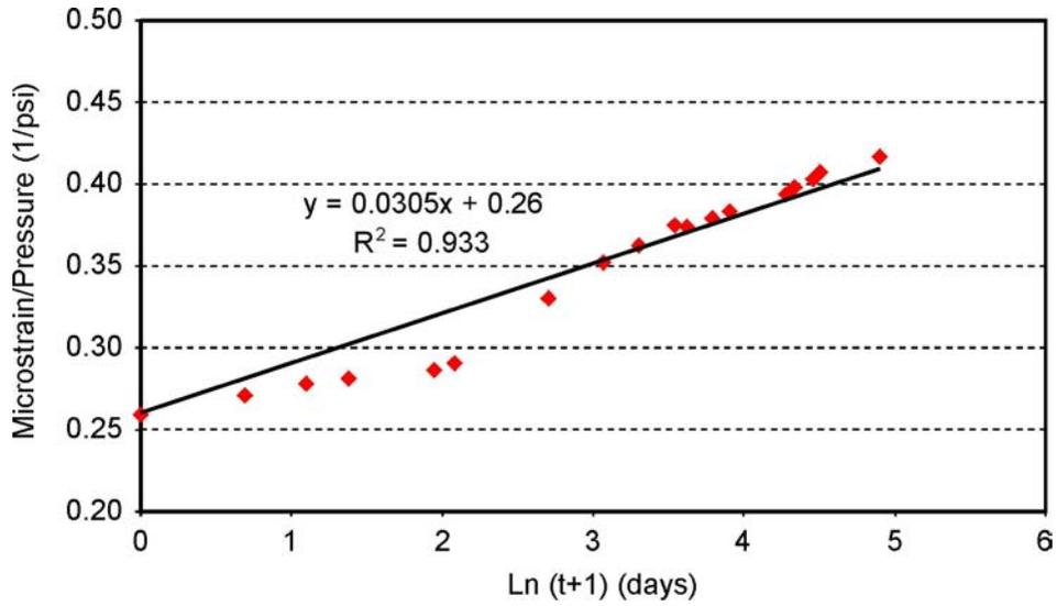
Figure 4. Creep Rate for Mattaponi Bridge Beams
