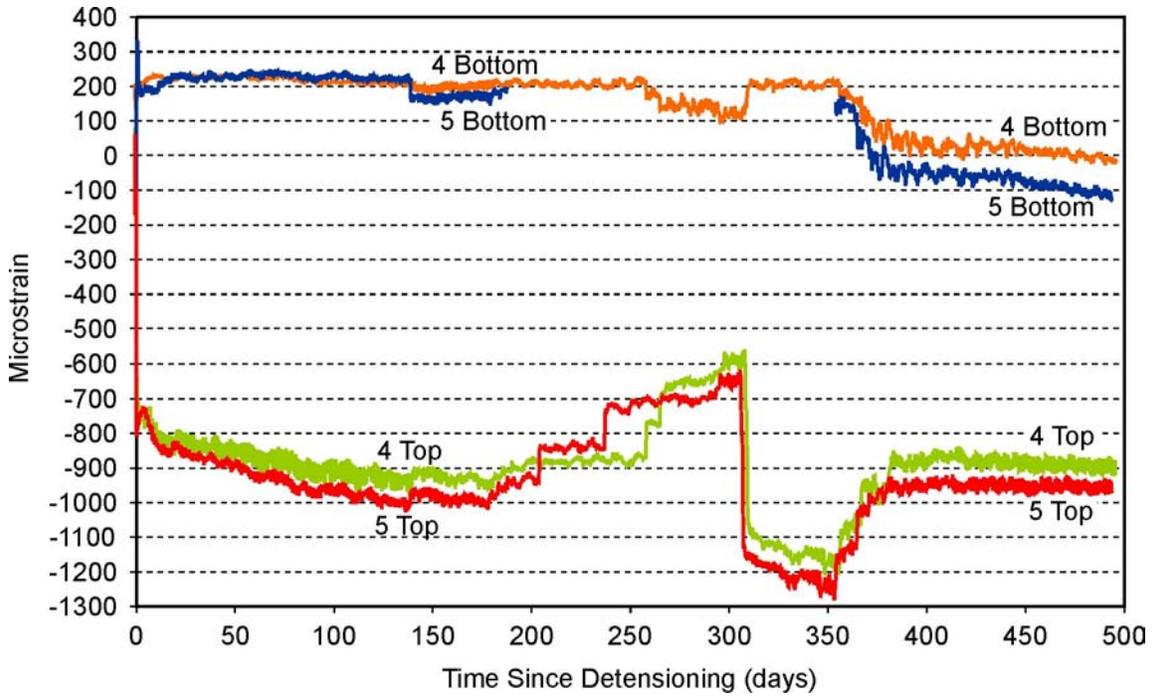
Figure 11. Strain Data for Pier Segment 34 of Pamunkey Bridge
