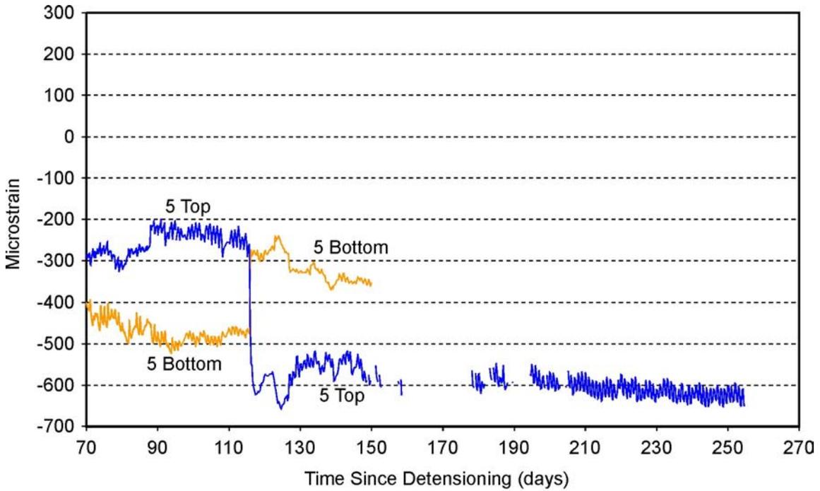
Figure 12. Strain Data for Beam HH5 of Pamunkey Bridge
