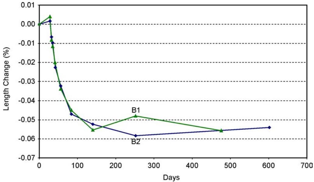
Figure 3. Pamunkey Deck Length Change Data for Moist-Cured Specimens
