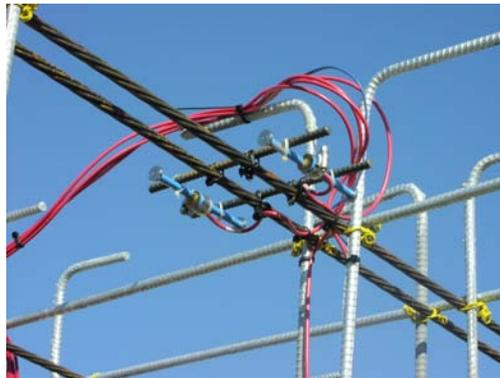
Figure 1. Vibrating Wire Gauges Located at Top of Beam
