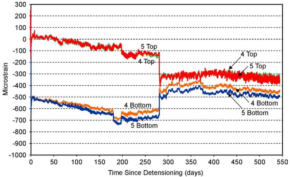
Figure 10. Strain Data for Span FF of Pamunkey Bridge
