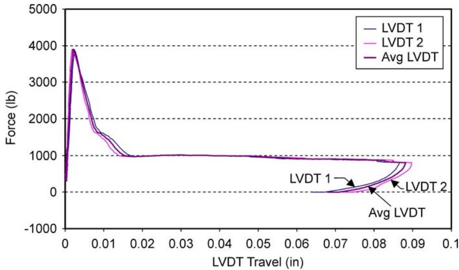
Figure 9. Example of Flexural Toughness Test of Beam with 0.3% Polymer Fibers
