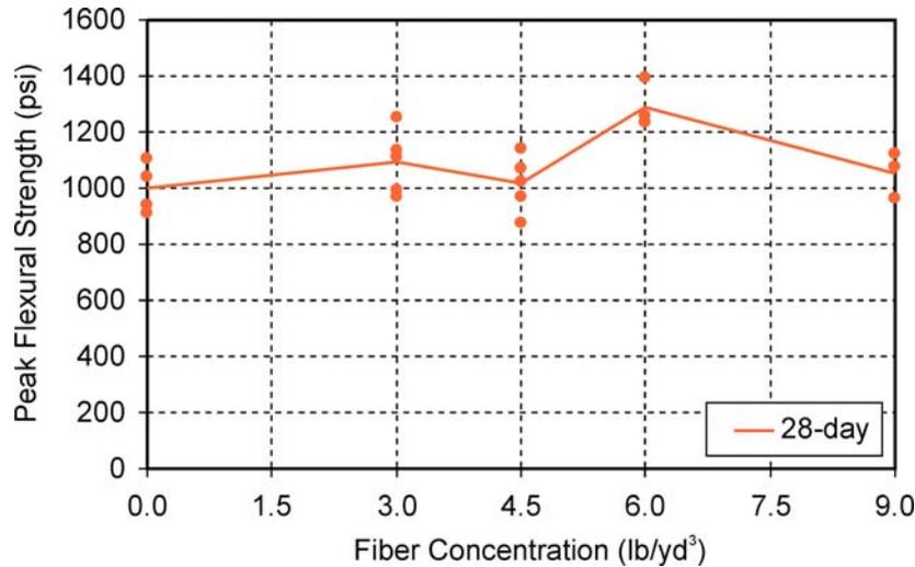
**Figure 5. 28-Day Flexural Strength Versus Fiber Concentration**
