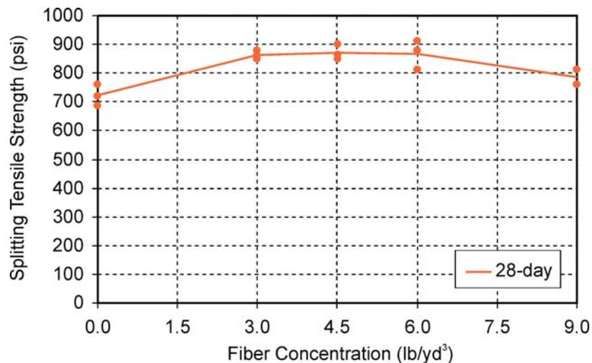
Figure 4. Splitting Tensile Strength Versus Fiber Concentration
