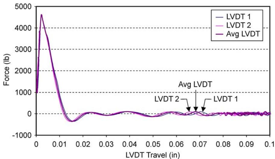
**Figure 8. Example of Flexural Toughness Test of Beam with No Fibers**
