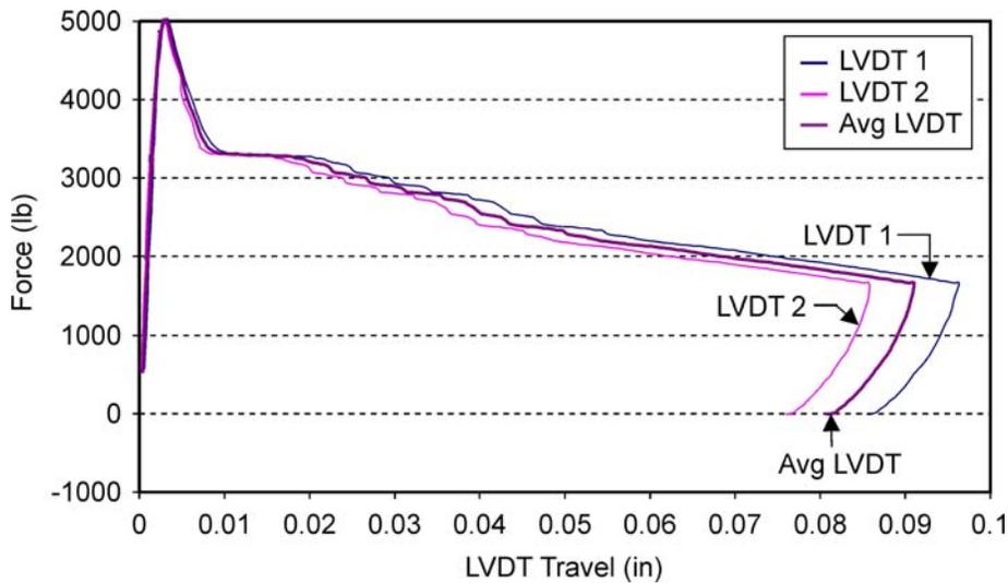
Figure 10. Example of Flexural Toughness Test of Beam with 0.5% Steel Fibers
