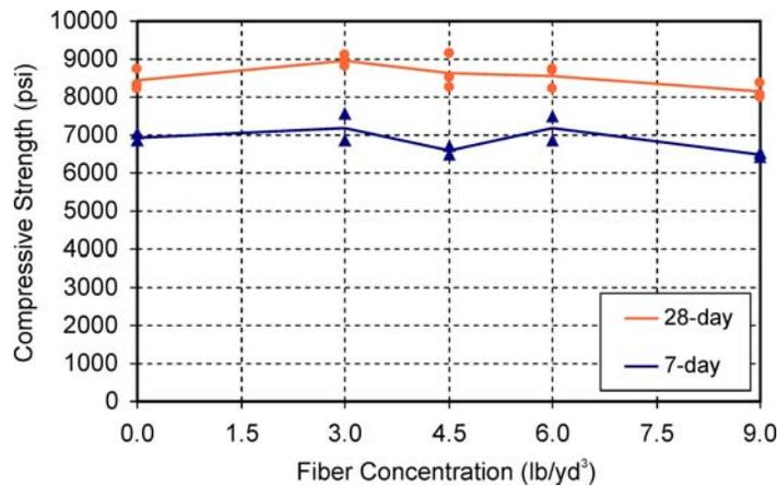
**Figure 2. Compressive Strength Versus Fiber Concentration**
