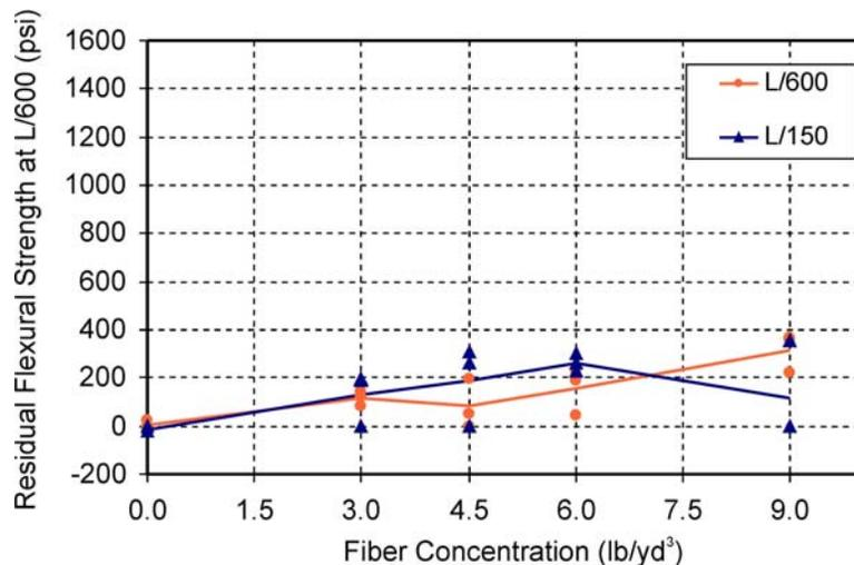
**Figure 6. Average Residual Strength Versus Fiber Concentration at a Deflection of L/600 (0.02 in) and L/150 (0.08 in) at 28 Days**
