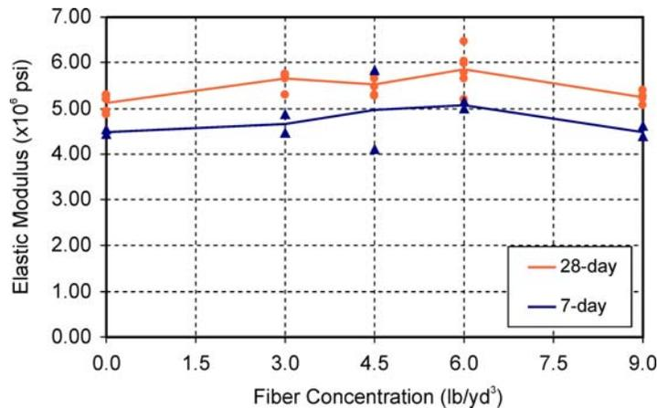
**Figure 3. Elastic Modulus Versus Fiber Concentration**
