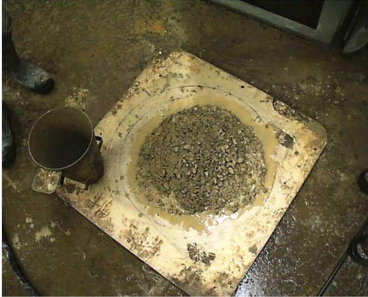
**Figure 1. Slump Flow Test of Concrete Exhibiting Excessive Bleeding and Segregation**
