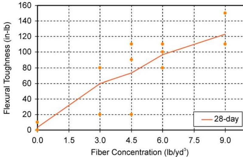
Figure 7. Flexural Toughness Versus Fiber Concentration at L/150 Deflection
