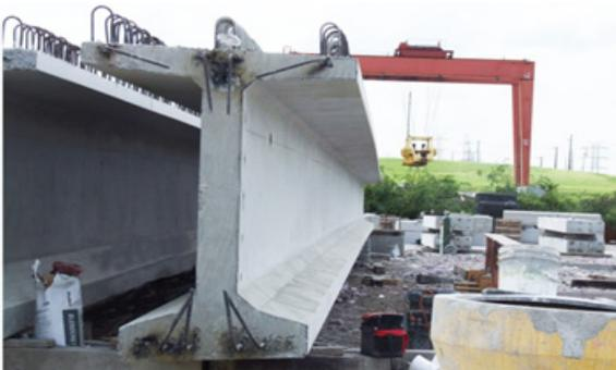
**The distinctive section of the bulb-T beam is evident in this photograph of the beam at the plant.**
