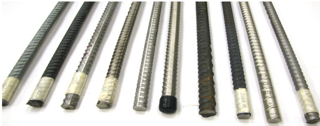
Various types of corrosion-resistant reinforcement bars that VTRC has tested, some of which are now routinely used by VDOT.
