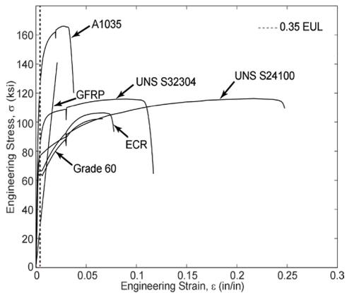
**Stress-strain diagrams for each bar type in phase I of the study**
