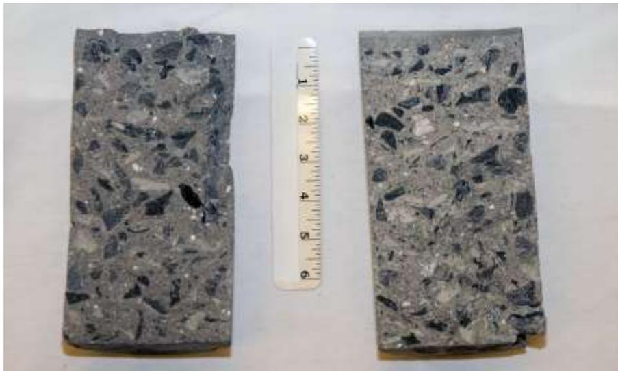
**Figure 3. Sample Concrete From Pier Caps.** The specimen on the left is from L2, which did not exhibit any halo and had a high strength. The specimen on the right is from L4, which showed marginal stability and had a lower strength than the other batches. The specimen has a paste layer 1/8 to 3/16 in deep on the top surface that was attributed to the marginal stability attested to by the slight halo.
