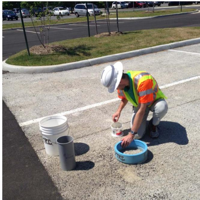
**Figure 3. Quality Check of Concrete at Stringfellow the Summer After Placement (Same Procedure Followed at Reston)**
