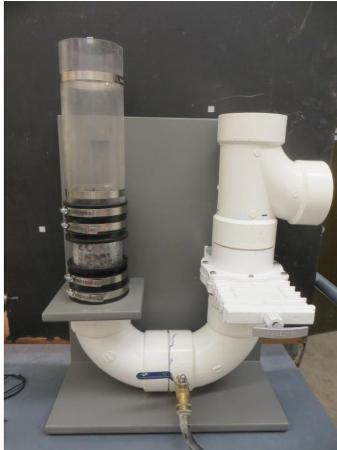
**Figure 2. Falling Head Permeameter for Hydraulic Conductivity**
