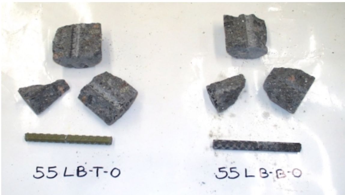
Figure 7. Tensile Bond Pullout Strength Specimens After Testing. Left , epoxy-coated bar; right , black bar.
