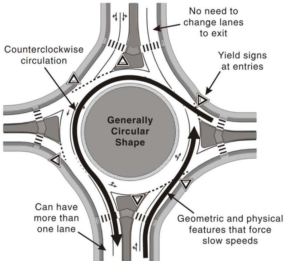
Modern roundabouts have demonstrated safety and operational benefits and should be considered as an alternative for intersection improvement projects. They can offer several advantages over signalized and stop controlled alternatives, including better overall safety performance, shorter delays, and shorter queues (particularly during off-peak periods), better management of speeds, and opportunities for community enhancement or aesthetic features.
