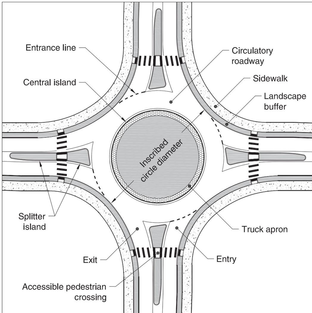
The principles and objectives of the geometric design of roundabouts are achieved using the general design process shown in Figure 6. In particular, performance checks are an important element of the design process and guidance found in the NCHRP Report 672, Section 6.7 should be followed to ensure the performance checks are completed appropriately, including sight distances.
