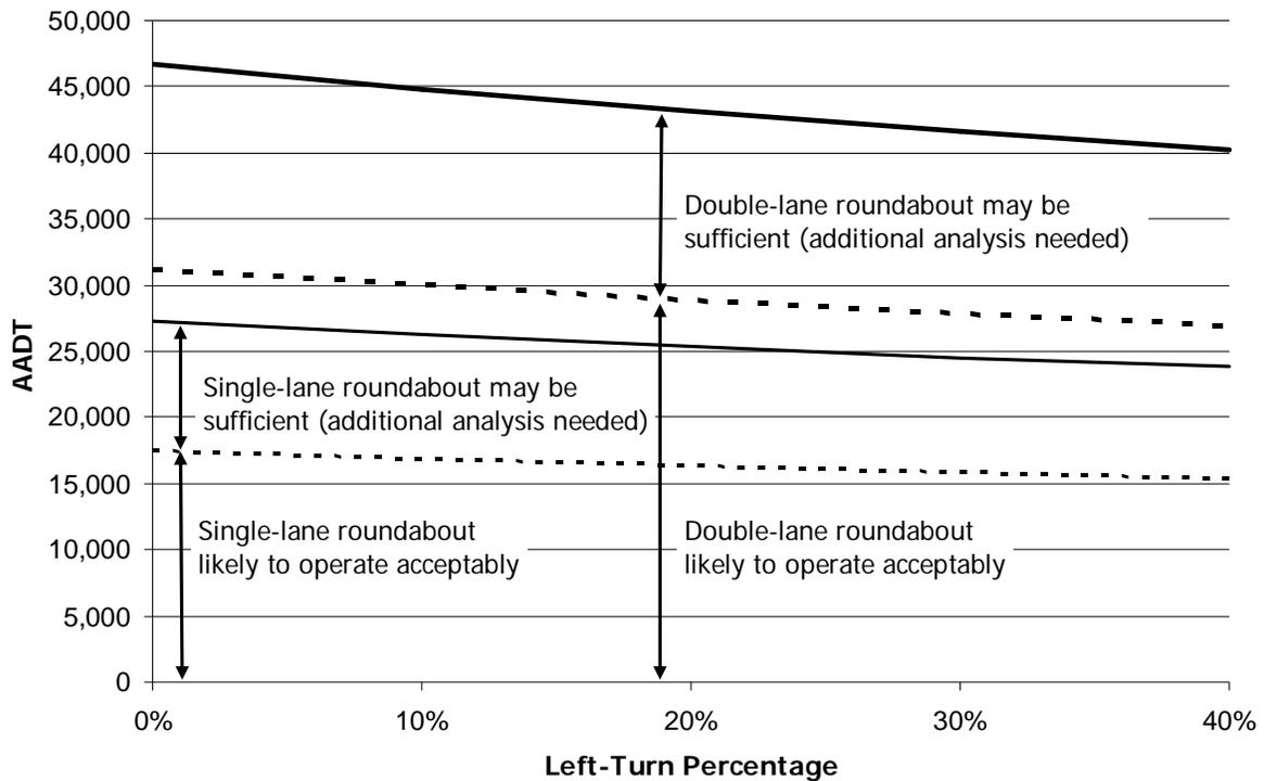
If the volumes fall within the ranges identified in Figure 4 where “additional analysis is needed,” a single-lane or two-lane roundabout may still function quite well, but a closer look at the actual turning-movement volumes during the design hour is required. The procedure for such analysis is presented in the 2010 *Highway Capacity Manual*, Chapter 21.
