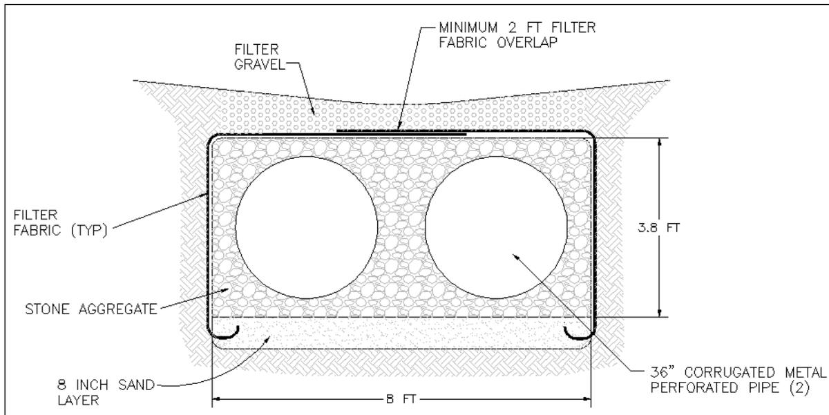
**Figure 8.3. Infiltration Trench Equipped with Perforated Pipes**
