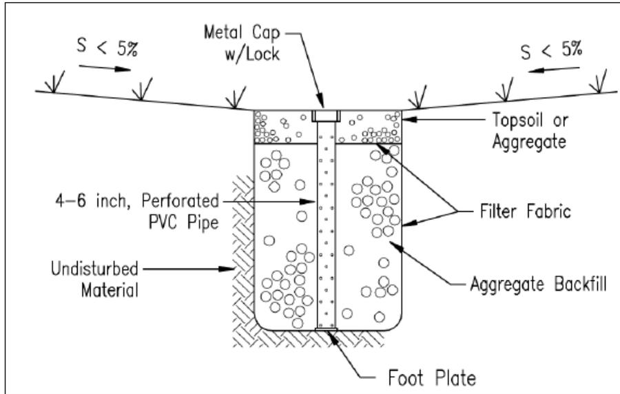
**Figure 8.1. Infiltration Trench Observation Well Configuration**
