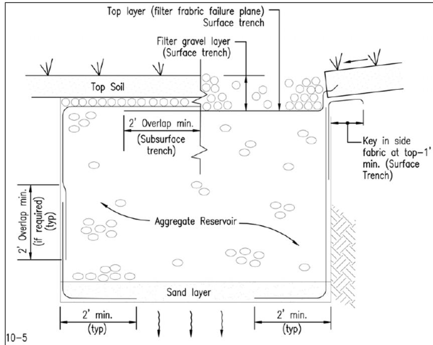
**Figure 8.2. Infiltration Trench Filter Fabric Installation**
