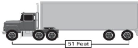
This 5 axle vehicle with 51 feet of axle spacing is allowed a maximum gross weight of 80,000 pounds.
