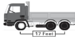
This 3 axle vehicle with 17 feet of axle spacing is allowed a maximum gross weight of 48,500 pounds.
