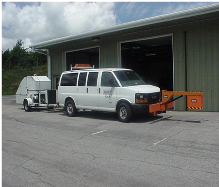
Figure 3 - Falling Weight Deflectometer
