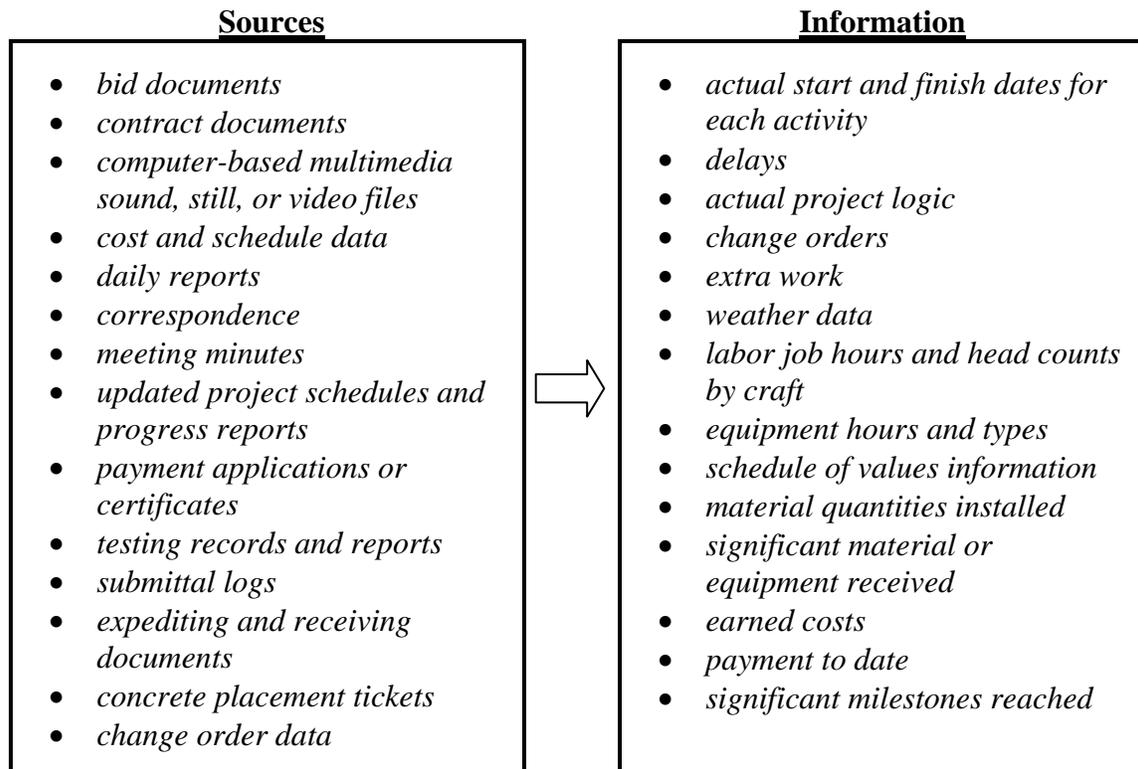
**Figure 3: Sources of Information used to Develop As-Built Schedule** [Knoke et al. 1996]
