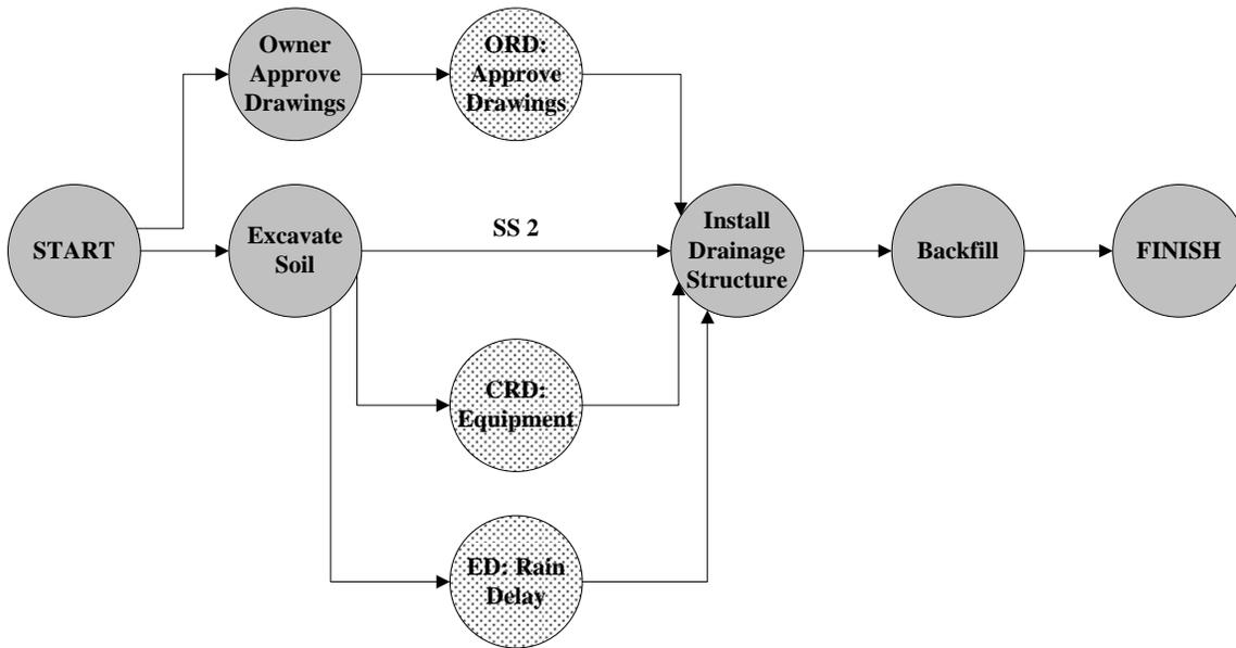
**Figure 6: As-Built CPM Network for Drainage Structure Example**
