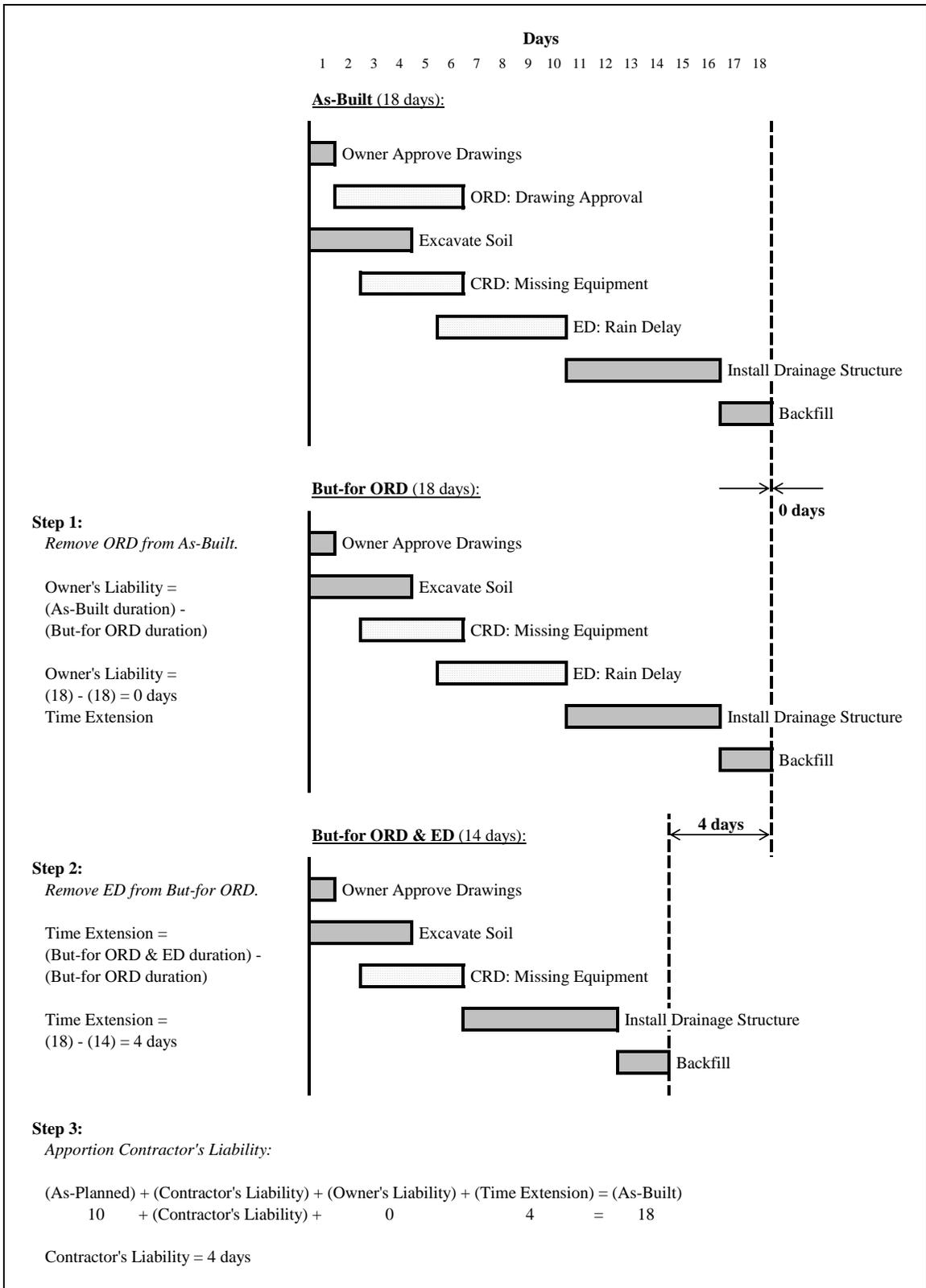
**Figure 18: Collapsed As-Built Schedule (But-for) Approach**
