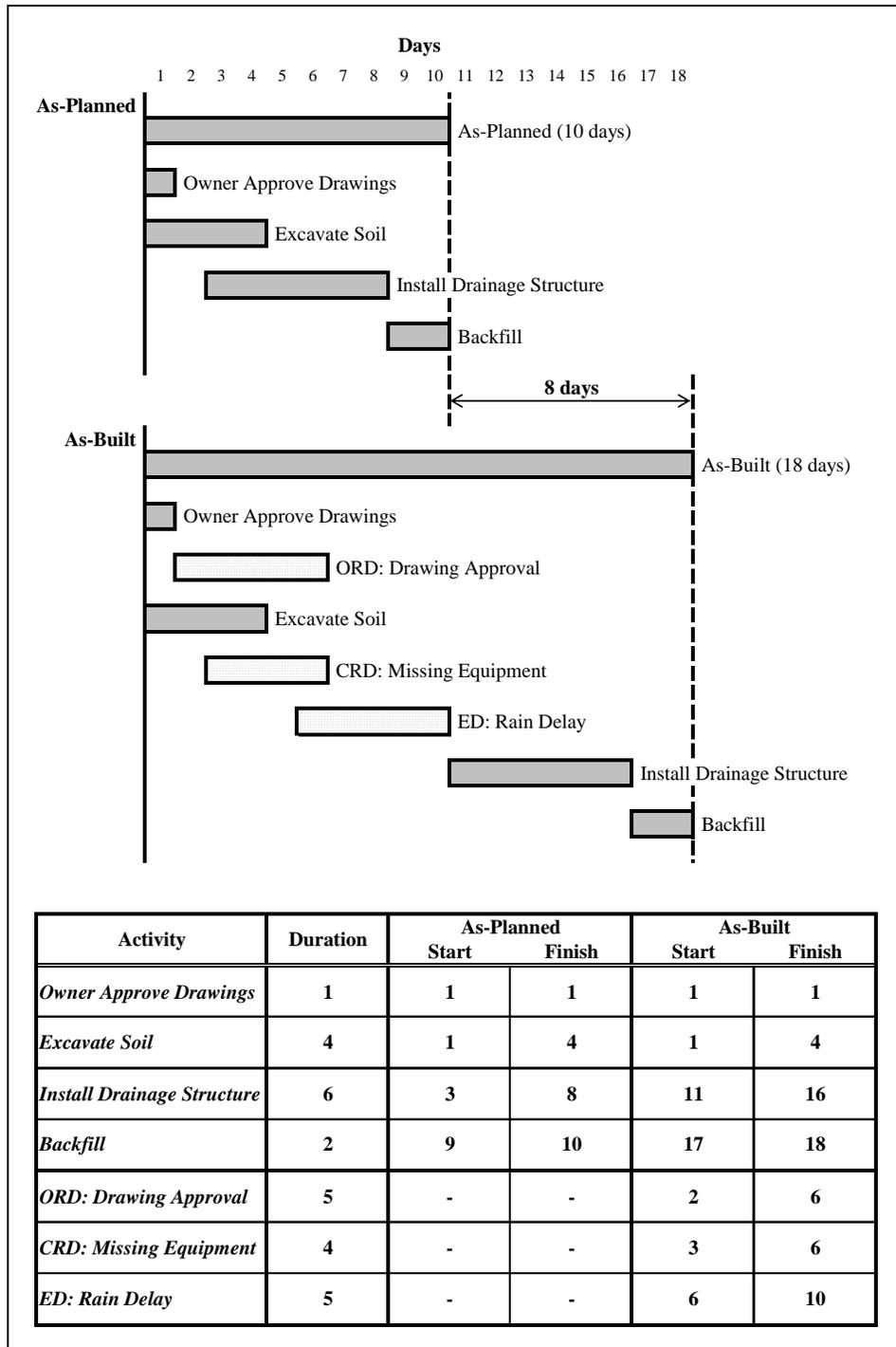
**Figure 12: Drainage Structure Example Bar Chart and Delays**
