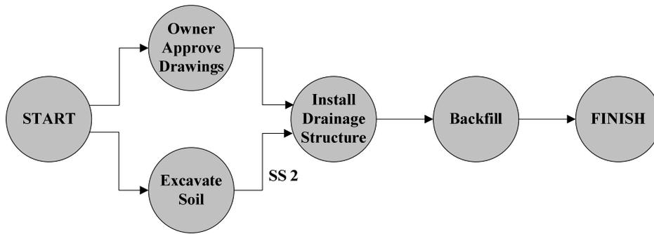
**Figure 5: As-Planned CPM Network for Drainage Structure Example**
