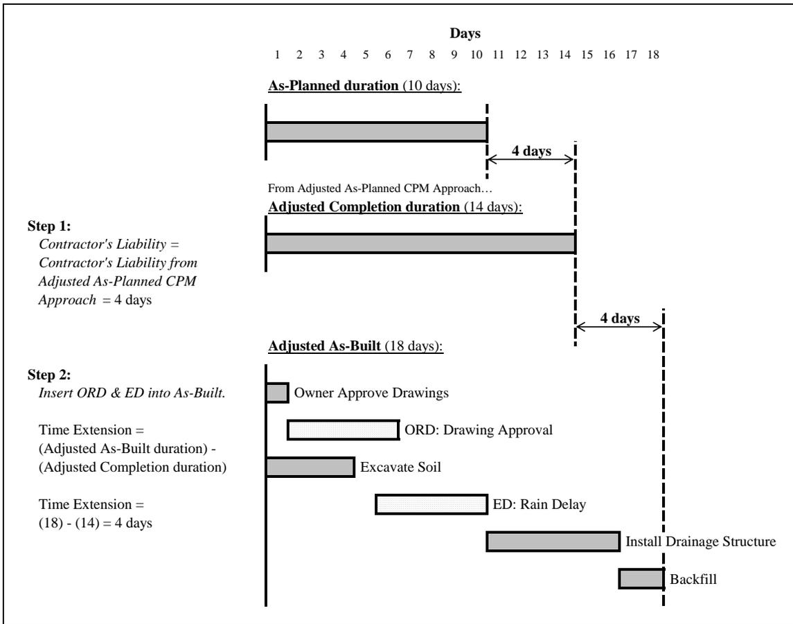
**Figure 17: Adjusted As-Built CPM Approach**
