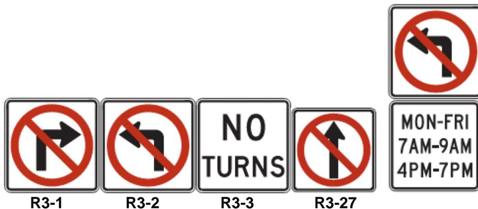
To illustrate the use of these signs, where a cut-through traffic issue is due to left-turning traffic, a sign restricting left turns could be installed. Typically, such issues occur at specific times of the day therefore, a regulatory sign restricting left turns would also include a supplementary plaque specifying the times it applies (as shown on above sign on the far right).
