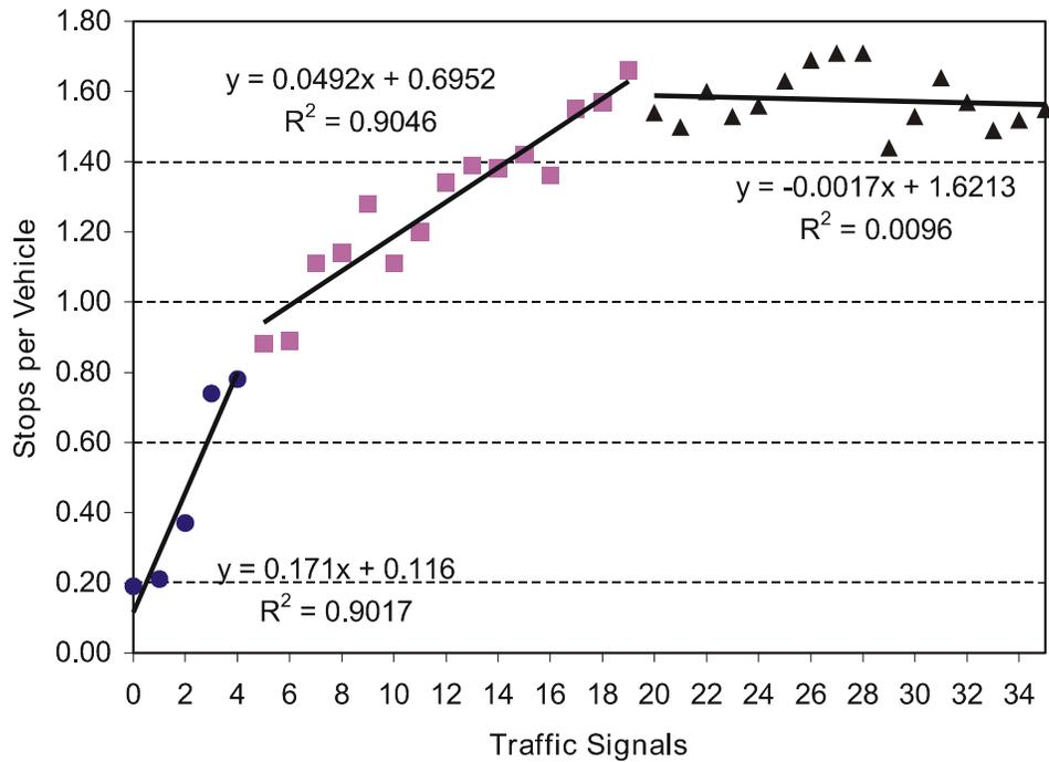
**Figure 4. Mainline Stops per Vehicle vs. Number of Traffic Signals (Route 17)**
