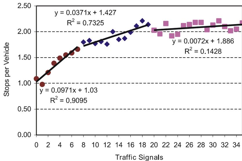
**Figure 6. Total Stops Per Vehicle vs. Number of Traffic Signals (Route 17)**
