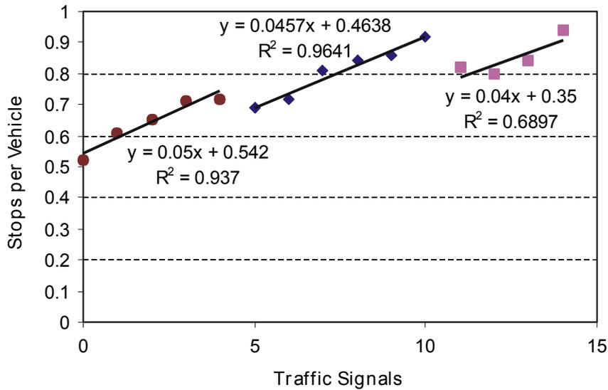
Figure 7. Total Stops Per Vehicle vs. Number of Traffic Signals (Route 250)
