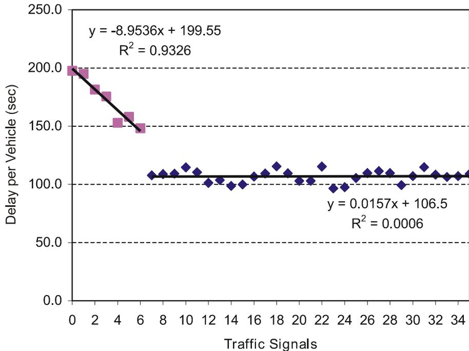
Figure 8. Total Delay per Vehicle vs. Number of Traffic Signals (Route 17)
