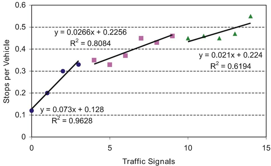
**Figure 5. Mainline Stops per Vehicle vs. Number of Traffic Signals (Route 250)**
