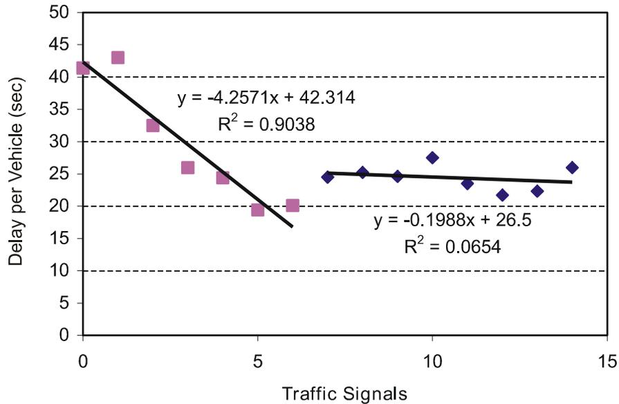
**Figure 9. Total Delay per Vehicle vs. Number of Traffic Signals (Route 250)**
