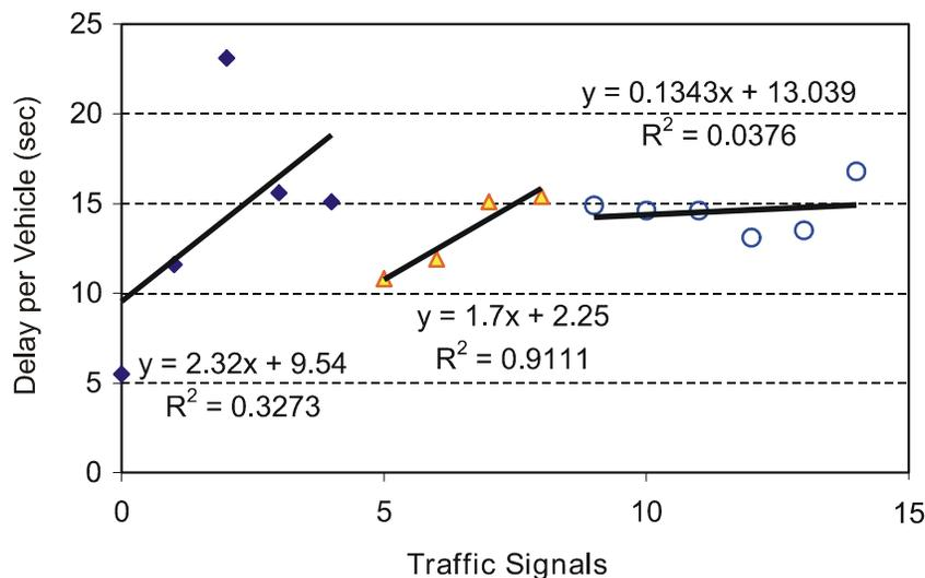
**Figure 12. Arterial Delay per Vehicle (Route 250)**
