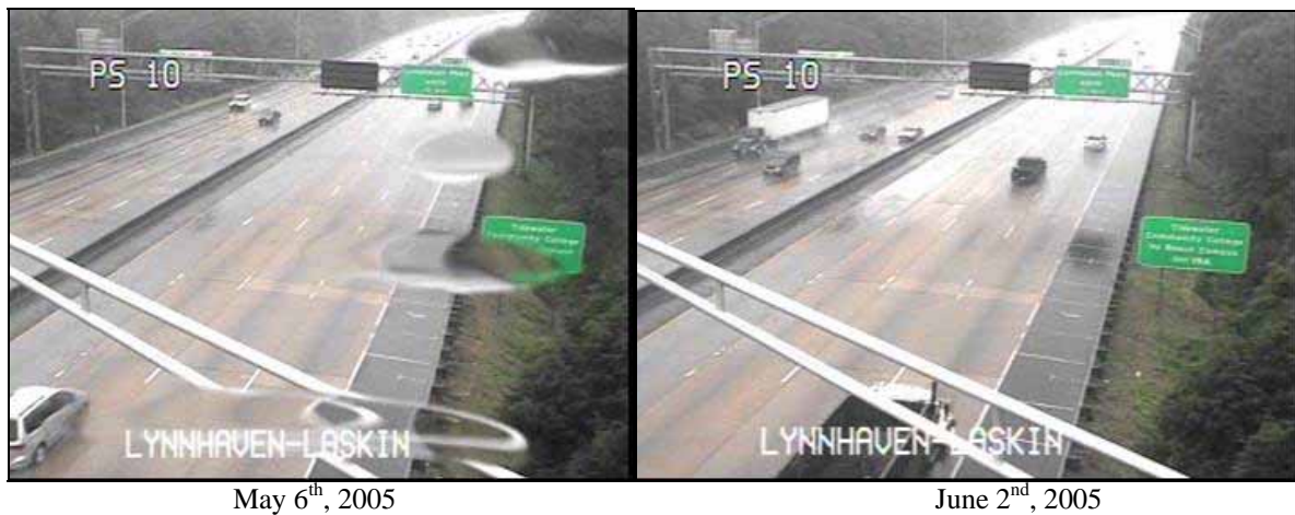
Figure 7. Rainy Day– Difference Between With/Without Rain Drops on CCTV Camera
