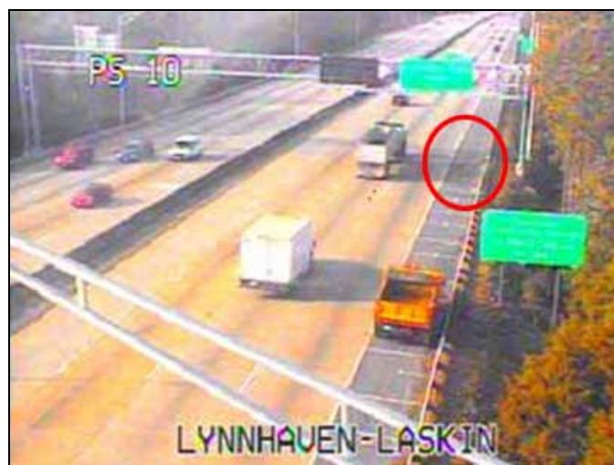
Figure 3. False Alarm Cause - Shadow Effect of Passing Vehicles
