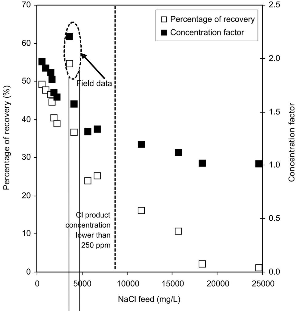
**Figure 6. Recovery Percentages of Product and Concentration Factor on Reject Streams at NaCl Feed Concentrations Tested**
