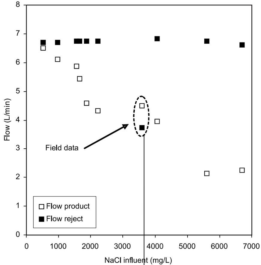
**Figure 11. Flows of Product and Reject as Function of NaCl Concentration on Feed During Low Concentration and Field Experiments**
