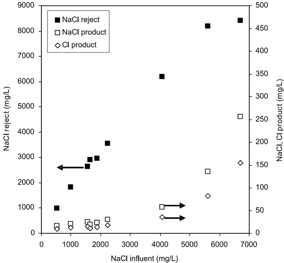
**Figure 3. Product and Reject NaCl Concentrations as Function of Feed NaCl Concentration**
