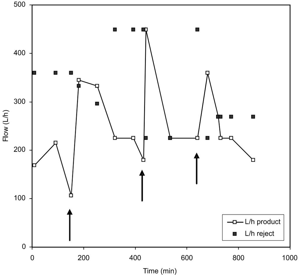
**Figure 8. Product and Reject Flows of Microfiltration Stage of Field Tests (arrows indicate timing of a cleaning procedure)**
