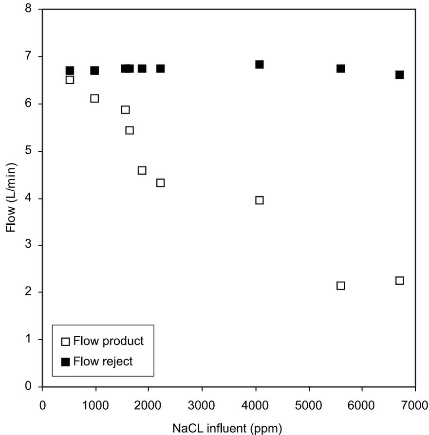
**Figure 4. Flows of Product and Reject as Function of NaCl Concentration on Feed During Low Concentration Experiments**
