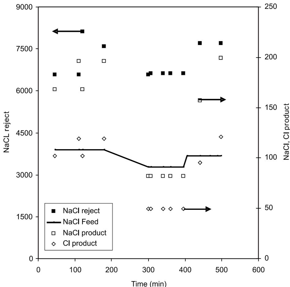
**Figure 9. NaCl Concentrations of Feed and Reject Streams and Chloride Concentration of Product Stream on Reverse Osmosis Stage in Field Experiments (arrows indicate axis to be used for data point types)**
