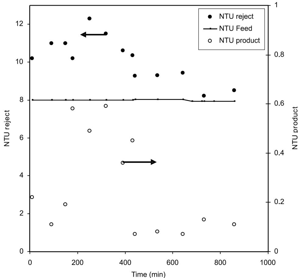
**Figure 7. Turbidity Reduction Resulting from Microfiltration Pretreatment (arrows indicate axis to be used for data point types)**
