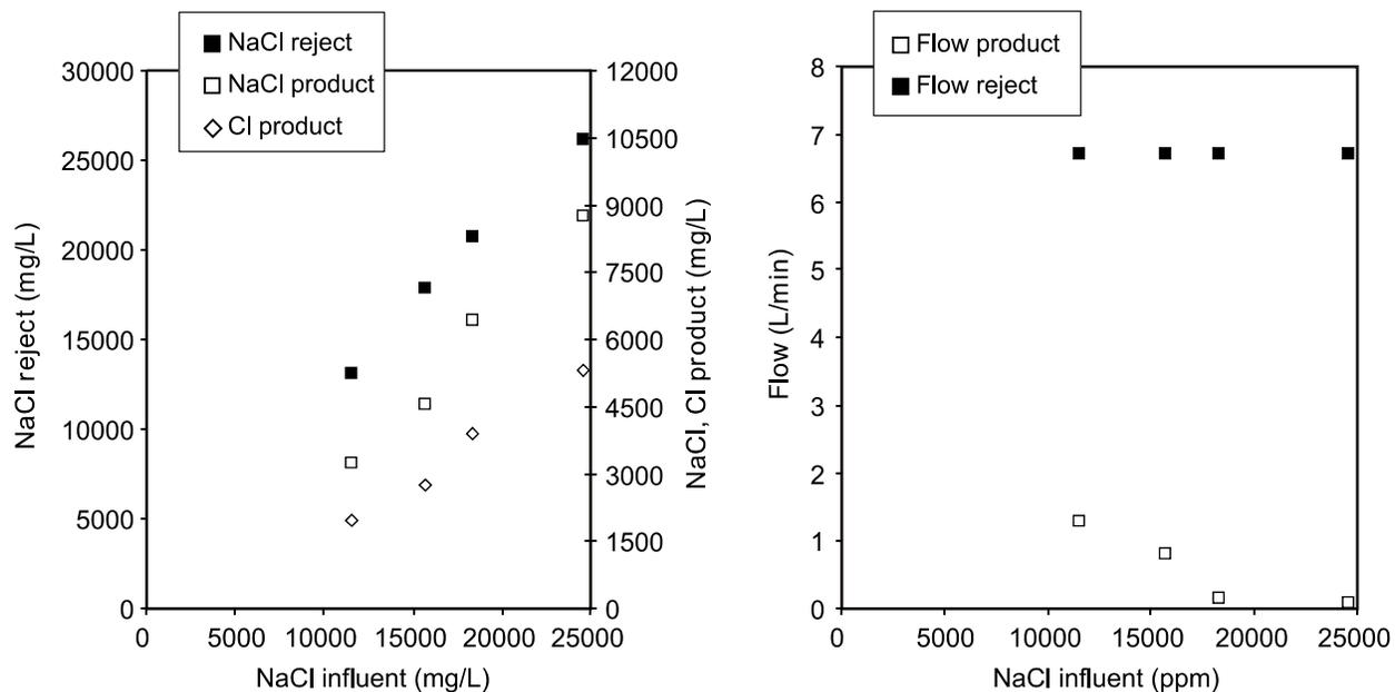
**Figure 5. (A) Product and Reject NaCl Concentrations as Function of Feed NaCl Concentration; (B) Flows of Product and Reject as Function of NaCl Concentration on Feed, During High NaCl Concentration Experiments**
