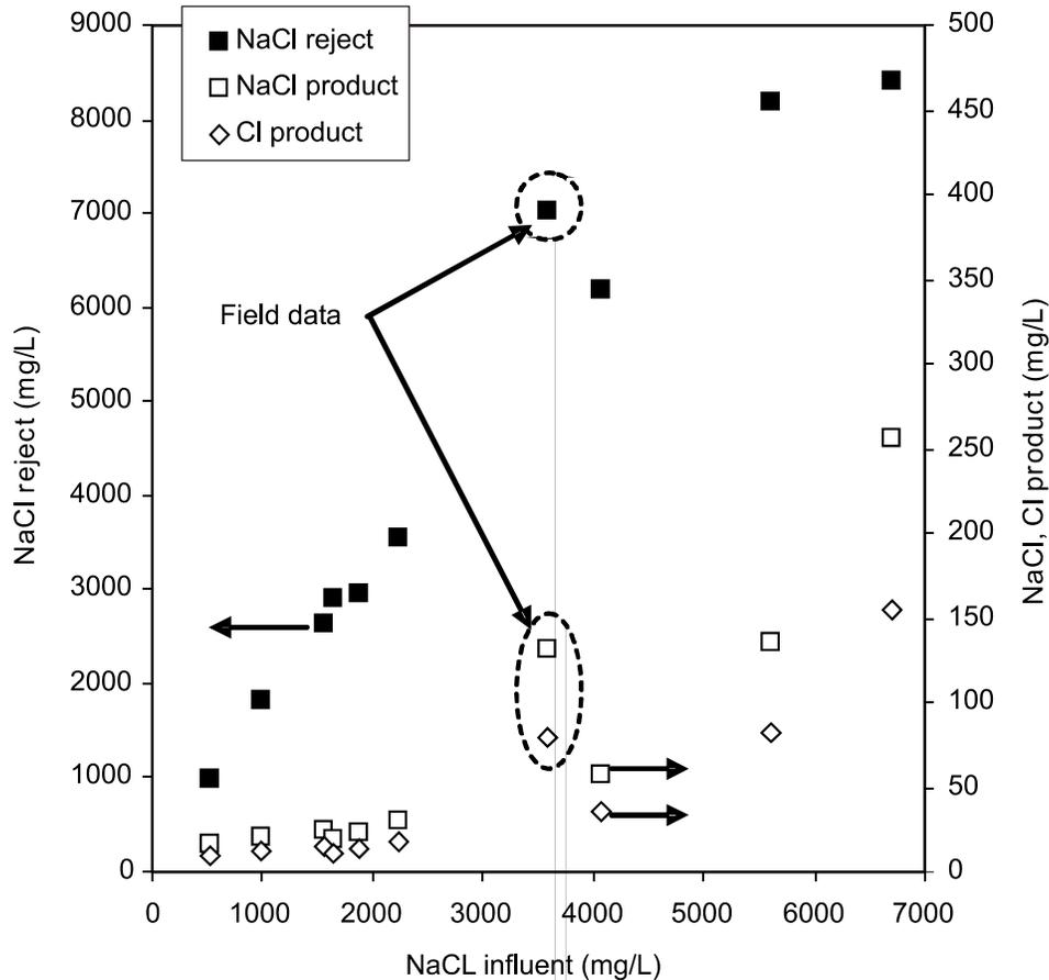
**Figure 10. Product and Reject NaCl Concentrations as Function of Feed NaCl Concentration During Low Concentration and Field Experiments (arrows indicate axis to be used for data point types)**
