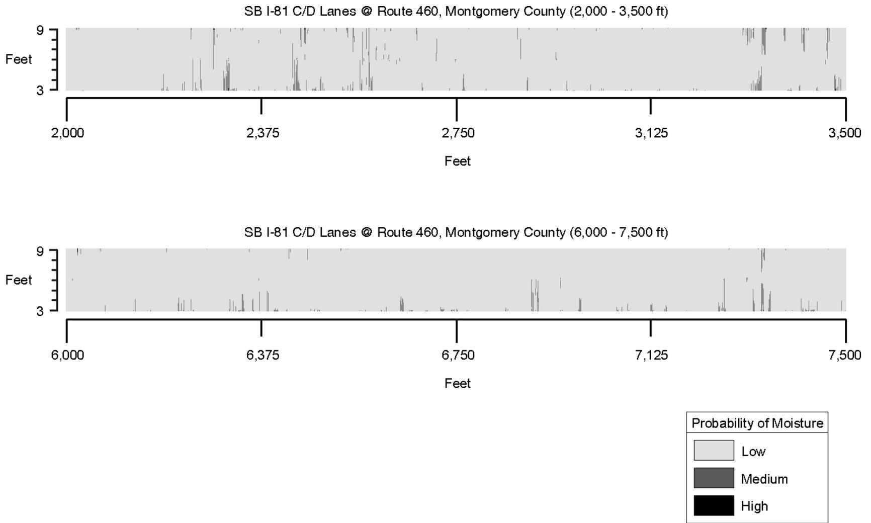
**Figure A-9. Normalized dielectric constant showing probability of moisture for portions of southbound I-81 collector/distributor lanes at Route 460 in Montgomery County**
