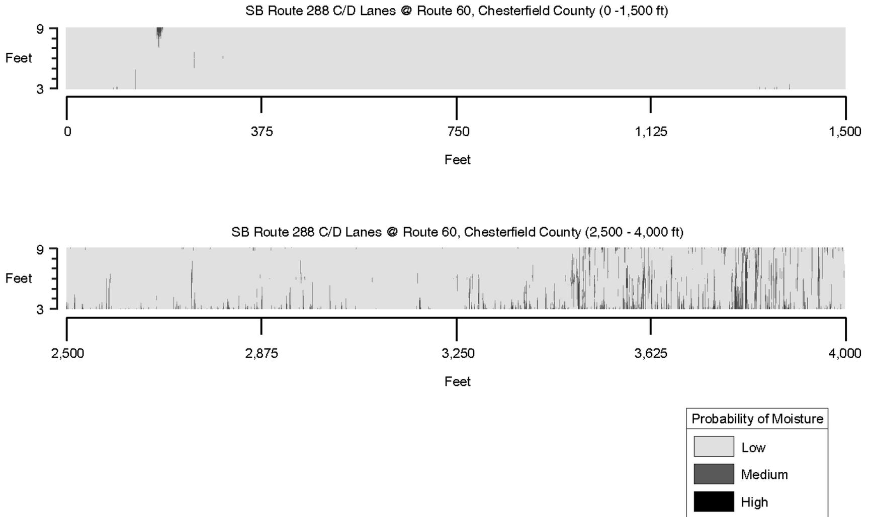
Figure A-2. Normalized dielectric constant showing probability of moisture for portions of southbound Route 288 collector/distributor lanes at Route 60 in Chesterfield County
