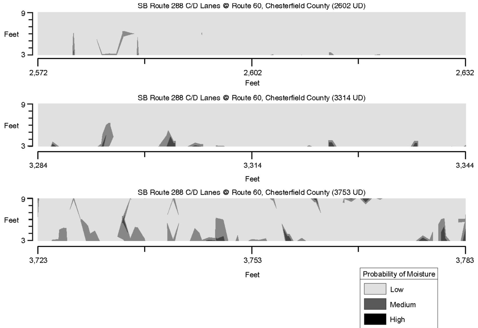
**Figure A-3. Detailed view of normalized dielectric constant showing probability of moisture for portions of southbound Route 288 collector/distributor lanes at Route 60 in Chesterfield County at locations of underdrain outlets**
