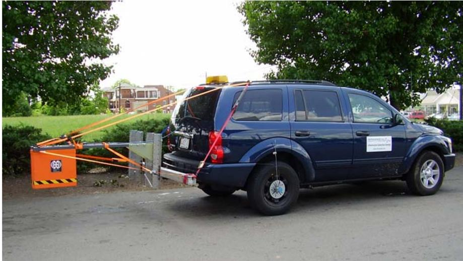
**Figure 2. Ground-Penetrating Radar Survey Vehicle**
