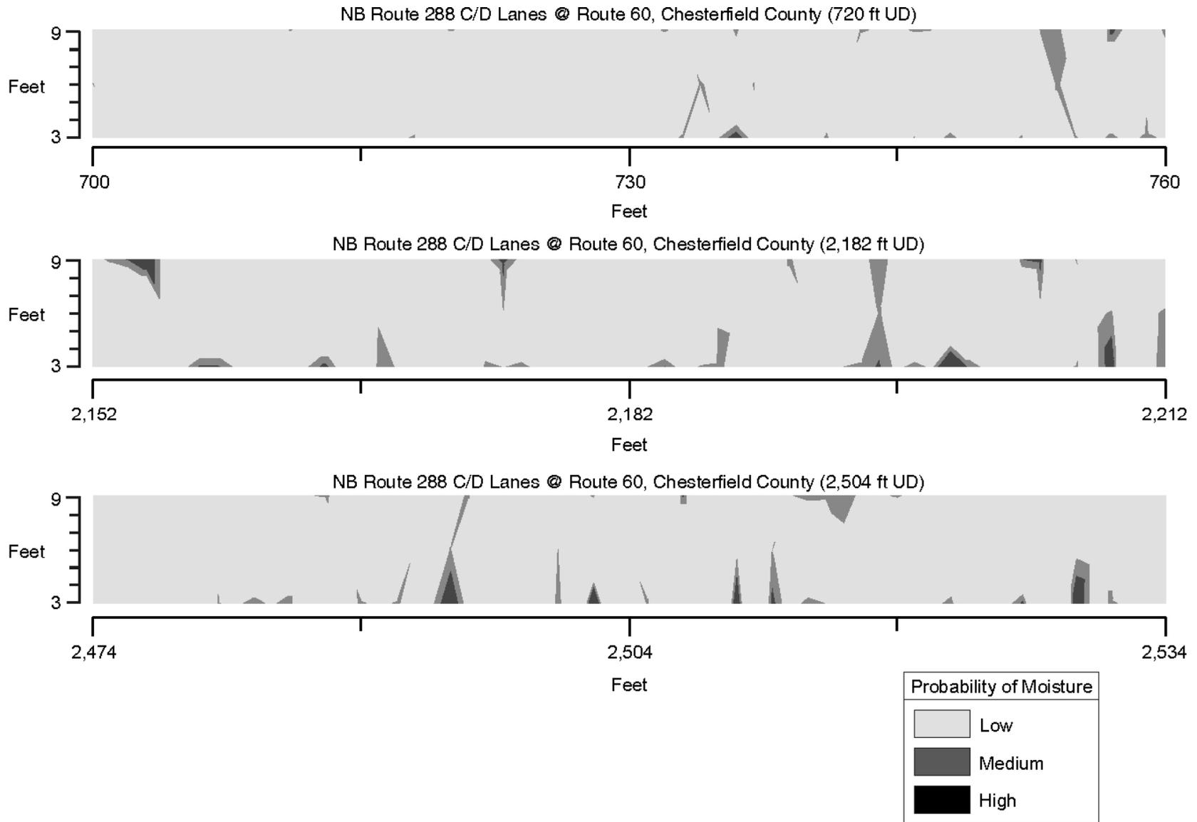
**Figure A-4. Detailed view of normalized dielectric constant showing probability of moisture for portions of northbound Route 288 collector/distributor lanes at Route 60 in Chesterfield County at locations of underdrain outlets**
