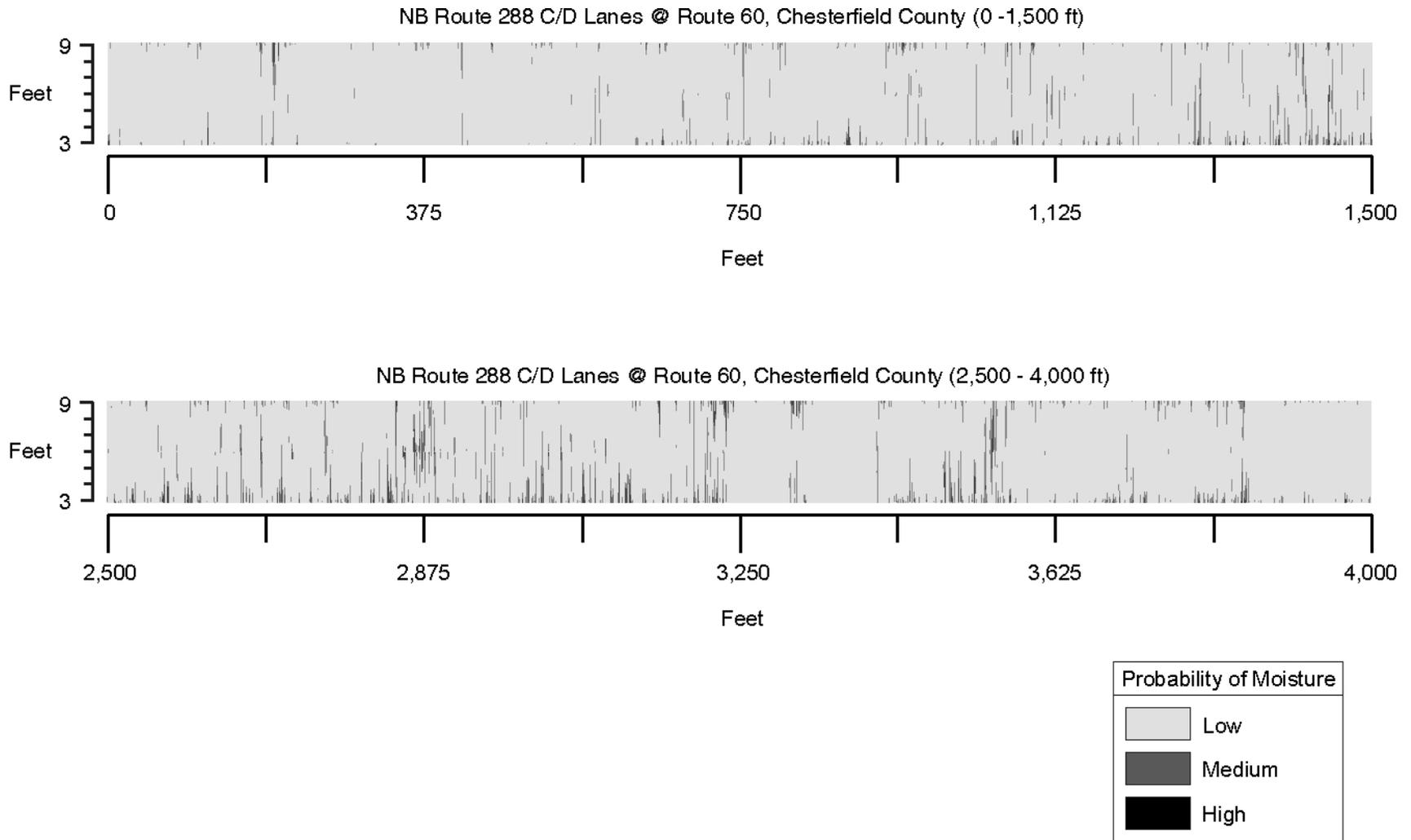
**Figure A-1. Normalized dielectric constant showing probability of moisture for portions of northbound Route 288 collector/distributor lanes at Route 60 in Chesterfield County**
