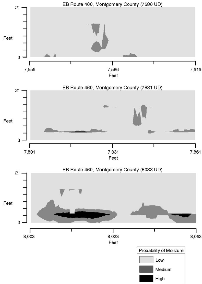
**Figure A-13. Detailed view of normalized dielectric constant showing probability of moisture for portions of eastbound Route 460 in Montgomery County at locations of underdrain outlets**
