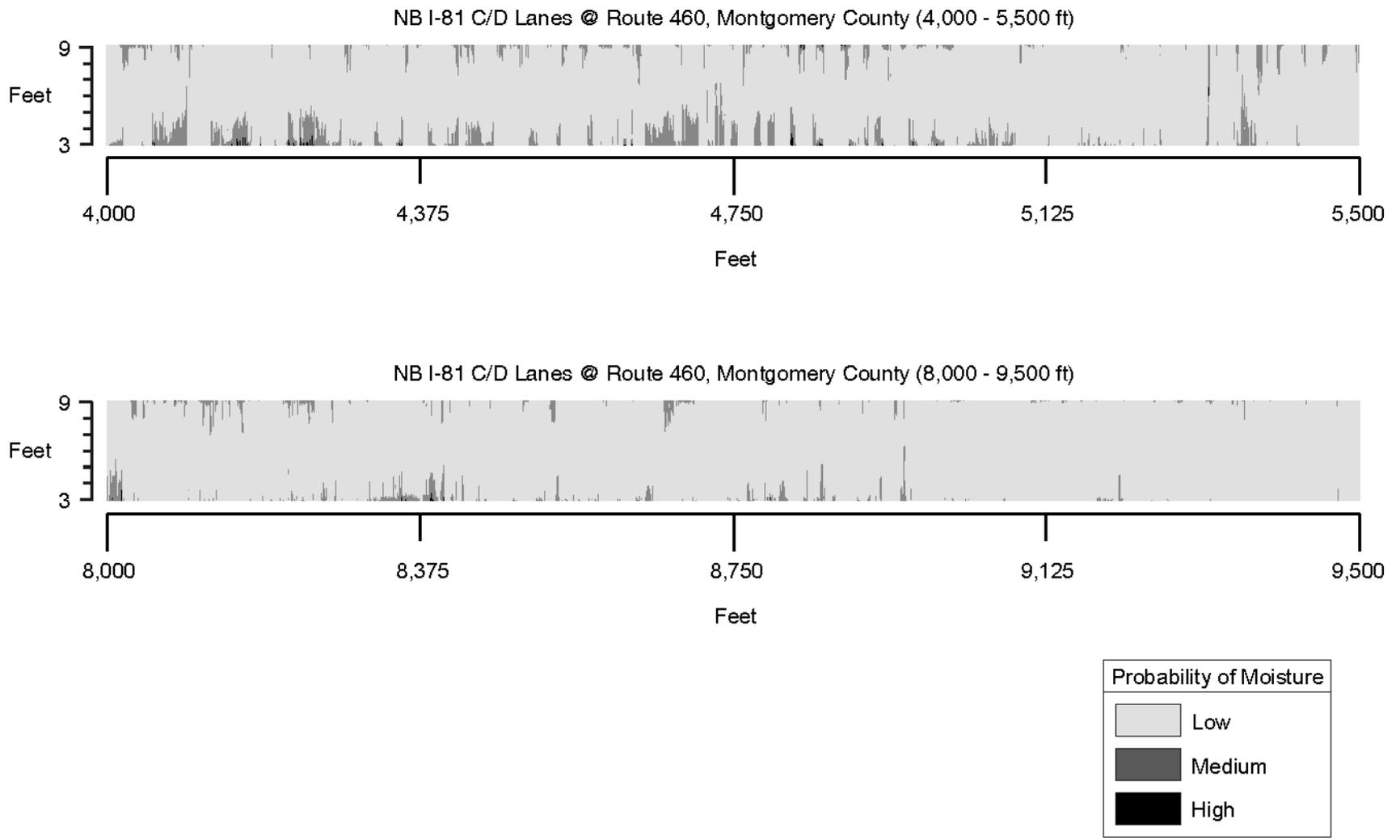
**Figure A-10. Normalized dielectric constant showing probability of moisture for portions of northbound I-81 collector/distributor lanes at Route 460 in Montgomery County**
