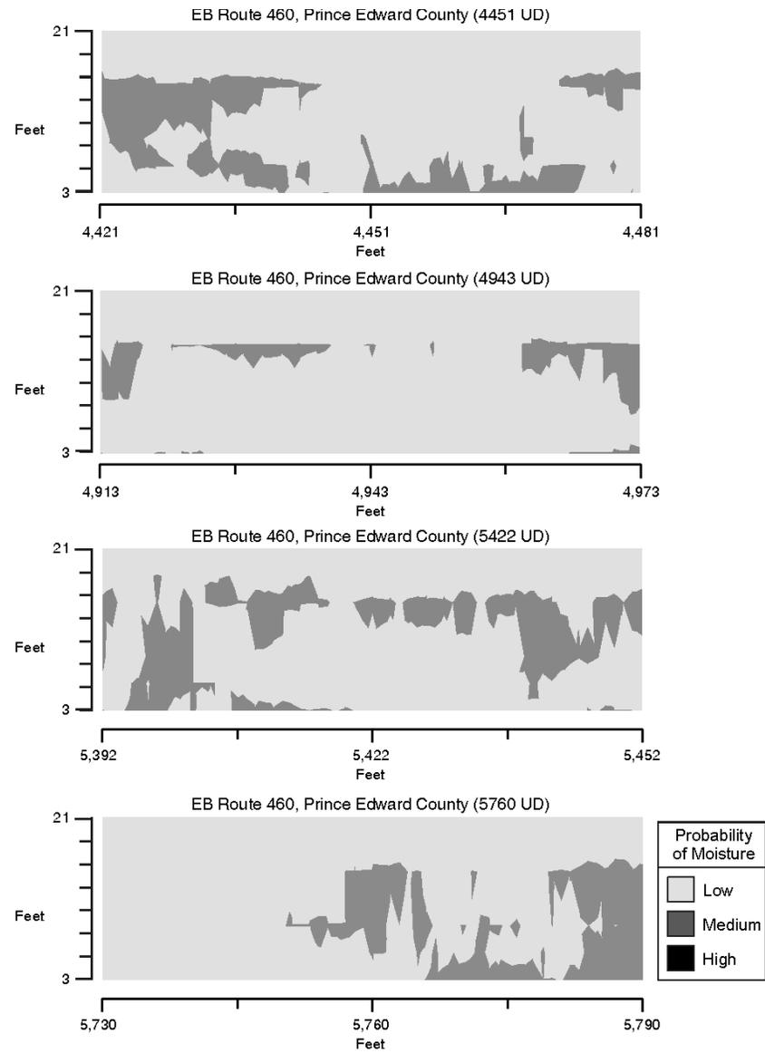
**Figure A-7. Detailed view of normalized dielectric constant showing probability of moisture for portions of eastbound Route 460 in Prince Edward County at locations of underdrain outlets.**
