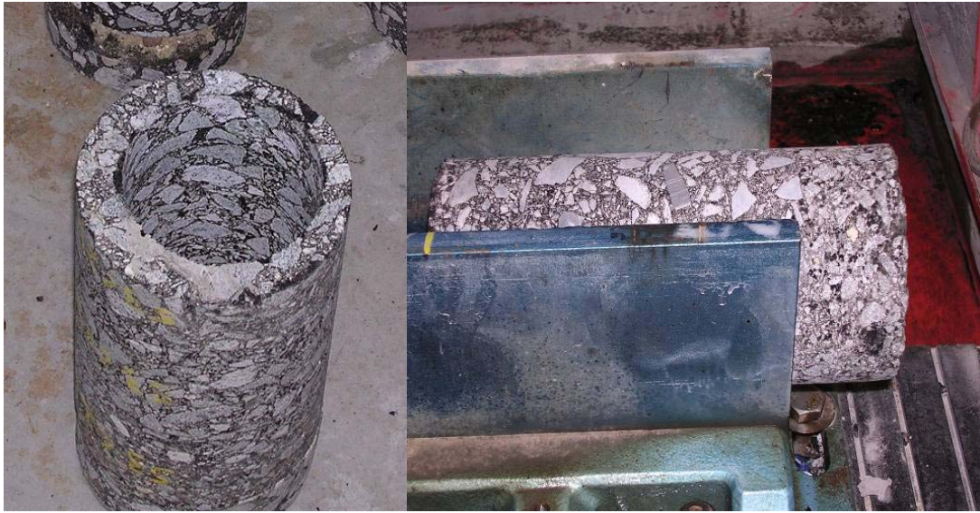
Figure 2. Coring and cutting of dynamic modulus specimens
