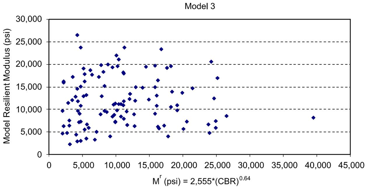
**Figure 4. Scatter Plot of Resilient Modulus Estimated from CBR and Model 3. Model 3 is recommended for use in the MEPDG**
