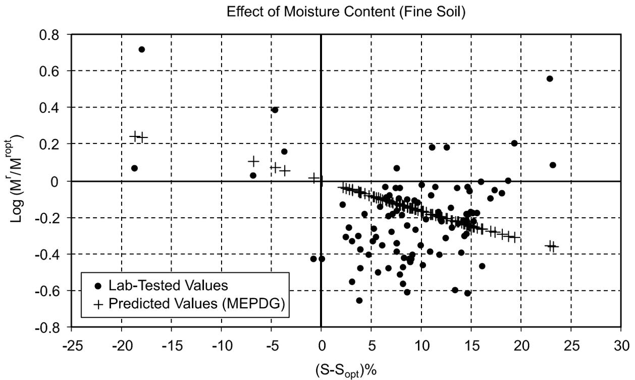
**Figure 3. Effect of Moisture Content on Soil Resilient Modulus. MEPDG = Guide for the Mechanistic-Empirical Design of New & Rehabilitated Pavement Structures.**
