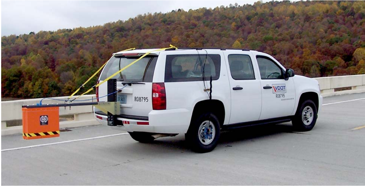
Figure 2. VDOT's Air-Launched Ground-Penetrating Radar System
