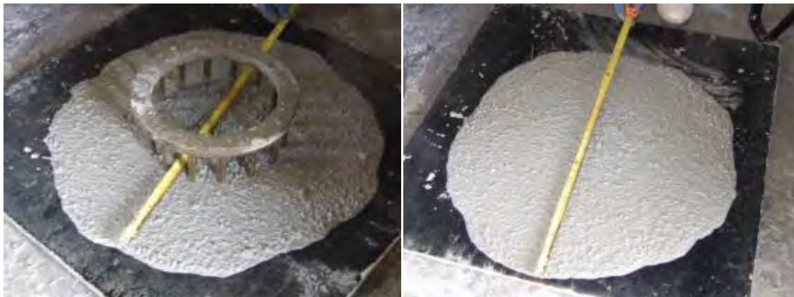
Figure 2. Slump Flow Tests of Self-Consolidating Concrete With and Without J-Ring
