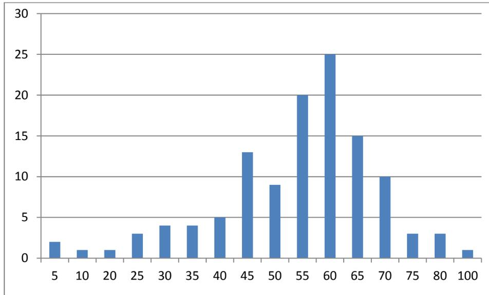
Figure 18. Speed of Vehicle Hitting TMA Before Crash. The speed data were rounded to multiples of 5.
