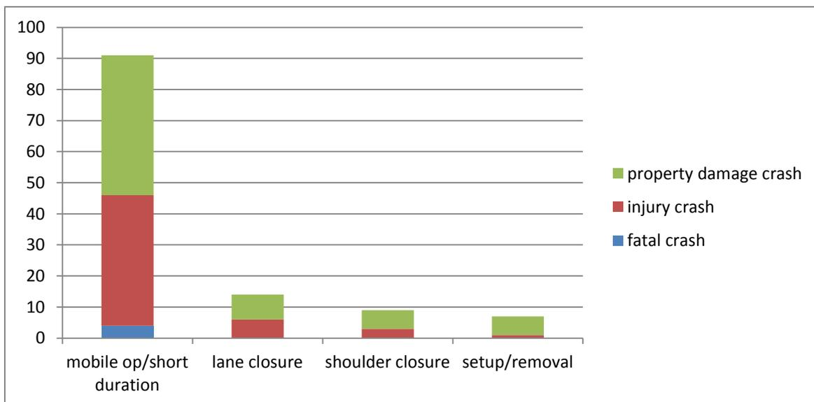
**Figure 7. TMA Crashes by Work Zone Type by Crash Severity**
