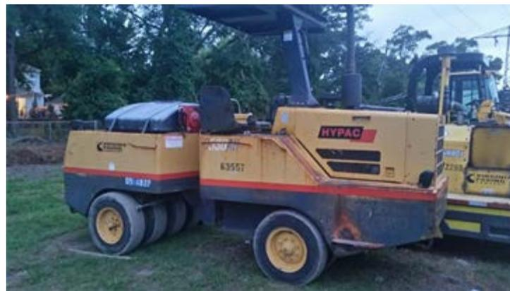
**Figure 8. Rubber Tire Roller**
