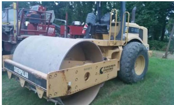
**Figure 9. Steel Drum Roller**
