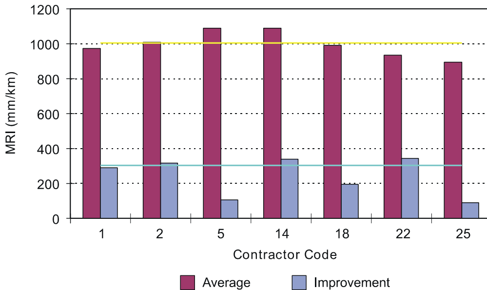
Figure 3. Contractor Performance for Interstate Resurfacing
