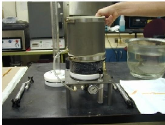
**Figure 2. Falling Head Permeameter**
